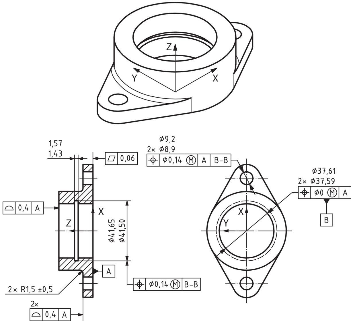
Figure 7 – Example of a mechanical engineering drawing
