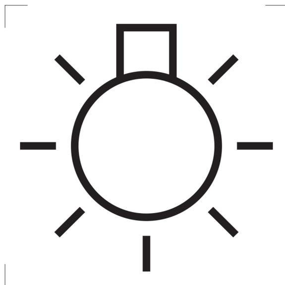
**Figure 8 – Example of a graphical symbol (IEC 60417-5012)**
