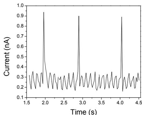
**Figure 4** Photocurrent of an individual carbon microcoil generated upon camera flash illustration at room temperature
