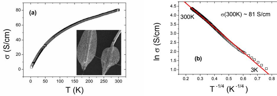
**Figure 3** Temperature dependence of electrical conductivity of an individual carbon microcoil, plotted as (a)  $\sigma(T)$  vs  $T$  and (b)  $\ln \sigma(T)$  vs  $T^{-1/4}$ . The inset shows an image of an isolated carbon microcoil with connected electrodes.
