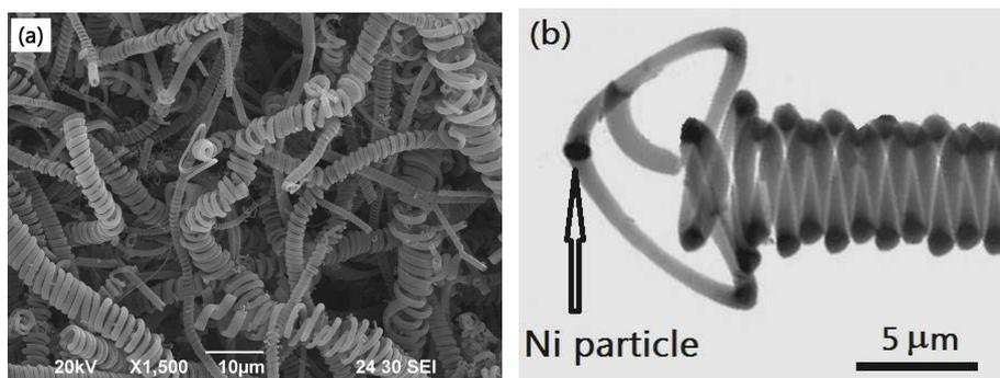
**Figure 1** (a) Typical SEM and (b) TEM images of the as-grown carbon microcoils. A Ni particle as a catalyst on an individual carbon microcoil can be seen clearly.
