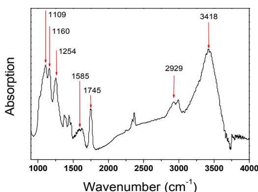
**Figure 2** IR spectra of the as-grown carbon microcoils
