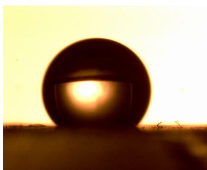
**Figure 5** Water contact angle of thin film of carbon microcoils is about  $135 \pm 1^\circ$ .
