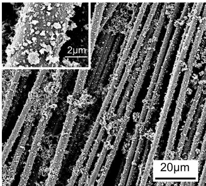
**Fig. 2.** SEM image of the aligned PANI/PMMA composite fibers. The inset shows the coated PANI nanostructures on the surface of a single PMMA fiber.
