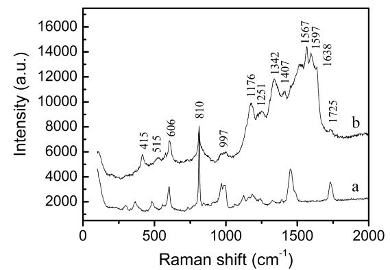
**Fig. 3.** Raman shifts of (a) pure PMMA fibers and (b) PANI/PMMA composite fibers.
