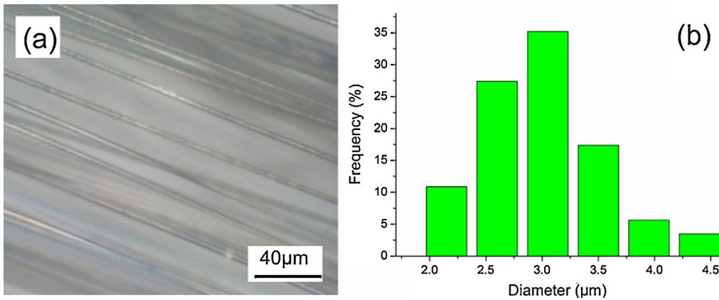
Fig. 1. (a) Photograph and (b) histogram showing the size distribution of aligned PMMA fibers.
