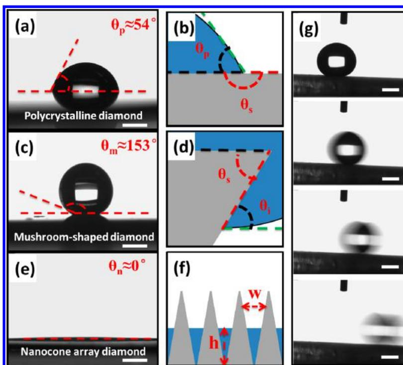
**Figure 5.** Static CAs of water on diamond surfaces and schematic of the wetting mechanism: (a, b) for polycrystalline diamond, (c, d) for mushroom-shaped structures, and (e, f) for a nanocone array. (g) Rolling process of a water droplet on mushroom-shaped structures. The scale bar is 1 mm.
