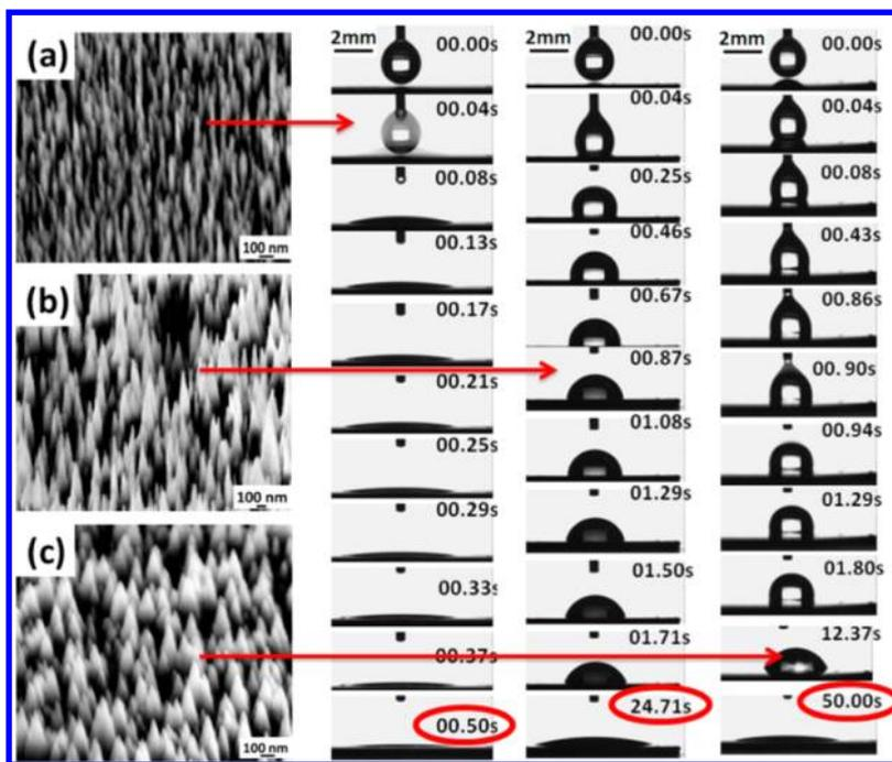
**Figure 6.** SEM images of diamond surfaces with different densities and profiles of nanocone arrays: (a) high density and sharp tip, (b) moderate density and moderate cone tip, (c) low density and blunt cone tip. The red arrows point to the process of water evolution on the corresponding surface.
