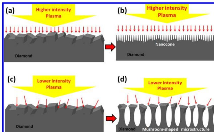
**Figure 3.** Schematic of the formation of diamond structures: (a) homogeneous etching of the polycrystalline diamond surface; (b) formation of nanocone diamond array structures; (c) selective etching of the polycrystalline diamond surface; and (d) formation of the arrayed mushroom-shaped diamond structures.
