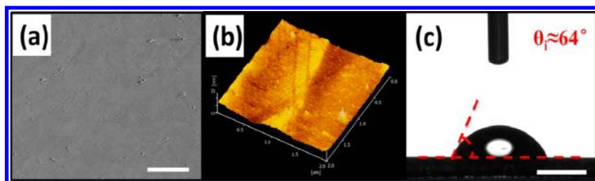
**Figure 4.** SEM and AFM images of the polished diamond surface and its wetting property: (a) SEM image with a scale bar of 5  $\mu\text{m}$ , (b) AFM image, and (c) static CA of water on the polished diamond surface with a scale bar of 1 mm.
