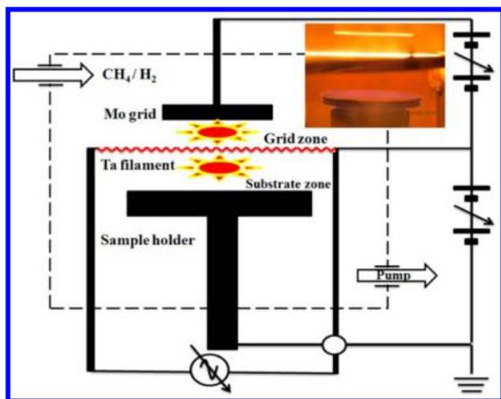
**Figure 1.** Schematic of the apparatus used to modulate the morphology of the diamond surface. The inset is a real plasma photograph of the grid-electrode region and substrate region.
