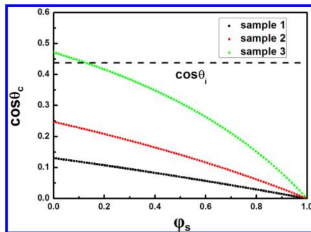
**Figure 7.** Change in the critical angle  $\cos \theta_c$  with  $\varphi_s$  for three kinds of diamond nanocone surfaces with different roughness values:  $r = 7.75$  (sample 1),  $r = 4.04$  (sample 2), and  $r = 2.12$  (sample 3), corresponding to different cone densities shown in Figure 6a–c, respectively. A black dashed line represents an intrinsic angle  $\cos \theta_i$  of 0.438.
