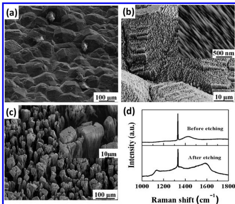
**Figure 2.** SEM images of the diamond surface: (a) the polycrystalline diamond surface used as a substrate, (b) the nanocone diamond structures, with an inset showing the details of the nanocones, and (c) the mushroom-shaped structures, with an inset showing the details of mushroom-shaped structures. (d) Raman spectra of the diamond film substrate before and after plasma etching.
