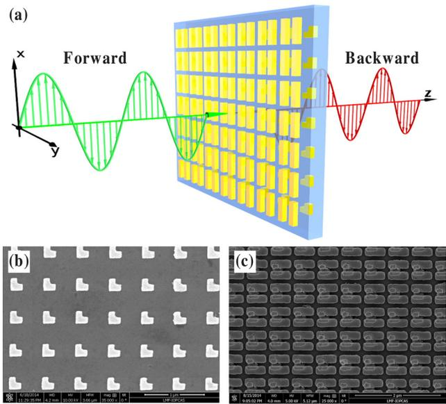
FIG. 1. (a) Schematics of the proposed two-layer hybrid metamaterial for  $x$ -polarized propagation in the forward and backward directions. (b) Scanning electron microscopy (SEM) image of the L-shaped metallic particle and (c) the double nano antenna.
