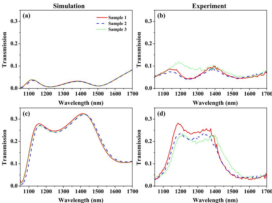
FIG. 5. (a) and (c) Simulated and (b) and (d) experimental transmission spectra of three relative translations for an  $x$ -polarized wave propagating along (a) and (b) the forward and (c) and (d) backward directions. Sample 1: the centers of the L-shaped metallic particle and the double nano antenna are aligned with each other; samples 2 and 3: the center of the L-shaped metallic particle has a 30 nm shift in  $x$ - and  $y$ -direction with that of the double nano antenna, respectively.
