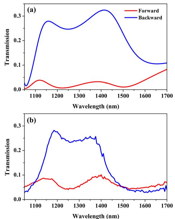
FIG. 3. (a) Simulated and (b) experimental transmission spectra of the ultrathin hybrid metamaterial for  $x$ -polarized wave propagating along the forward and backward directions.
