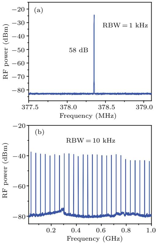
Fig. 3. (a) RF spectrum at the fundament beat note with the resolution bandwidth of 1 kHz. (b) RF spectrum at 1 GHz wide-span range with the resolution bandwidth of 100 kHz.
