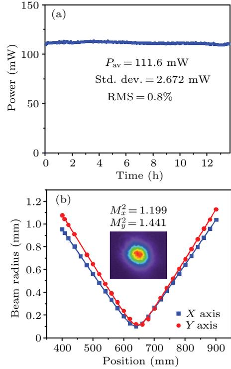
Fig. 4. (a) The power stability of the mode-locked Yb:LYSO laser. (b) The  $M^2$  factor measurement result and the profile of the laser output beam (inset).
