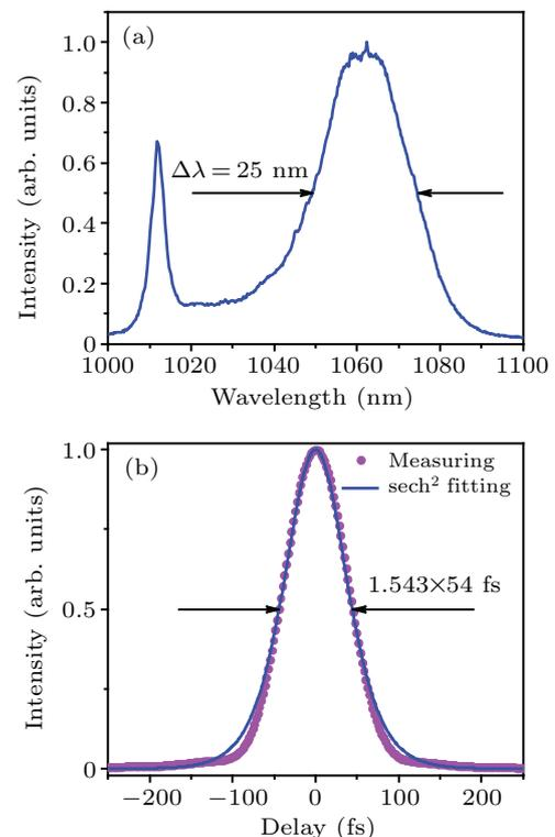
Fig. 2. (a) Measured optical spectrum of the mode-locked pulses. (b) Corresponding auto-correlation trace of the experimental data (dots) and the  $\text{sech}^2$ -fitting curve (solid).
