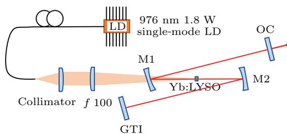
Fig. 1. Schematic diagram of the LD pumped KLM Yb:LYSO laser.
