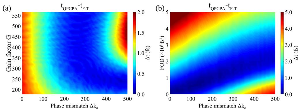
FIG. 5.  $\Delta t = t_{\text{QPCPA}} - t_{\text{F-T}}$  changes by varying the phase mismatch and (a) gain factor or (b) FOD, respectively. The Fourier-transform limit  $t_{\text{F-T}}$  is calculated with the corresponding QPCPA output spectrum.  $\alpha_{i0} = 8 \text{ cm}^{-1}$  and  $z = 10 \text{ mm}$ .
