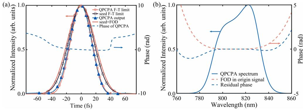
FIG. 4. The normalized signal pulse intensities and corresponding phase in the (a) temporal and (b) spectral region. The GDD of the QPCPA output is compensated, while the TOD is not compensated. The initial FOD is  $3 \times 10^5 \text{ fs}^4$ , gain factor  $G = 320.347 \text{ m}^{-1}$ ,  $\Delta k_0 = 298.81 \text{ rad/m}$ , and  $\beta_1 = -1.098 \text{ fs/mm}$ .  $\alpha_{i0} = 8 \text{ cm}^{-1}$  and  $z = 10 \text{ mm}$ .
