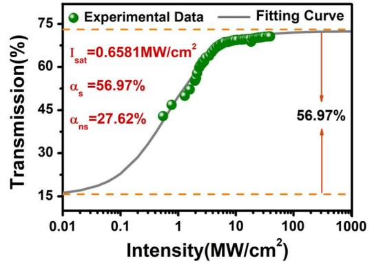
Fig. 1. Nonlinear optical transmission of CoOF-SA.
