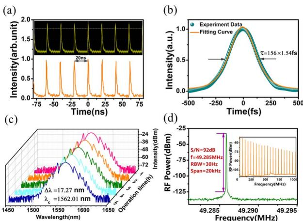
Fig. 3. (a) The pulse sequence. (b) The autocorrelation trace. (c) The spectra. (d) The RF spectrum.
