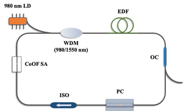
Fig. 2. Schematic diagram of high-stability MLFL cavity with CoOF SA.
