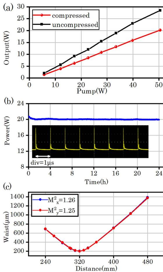
Fig. 5. (a) Dependence of output power versus the pump power for the main amplifier; (b) measured power stability and pulse train; (c)  $M^2$  value of this NCPA system.
