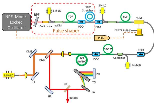
**Fig. 1.** Schematic of the NCPA system. BPF, bandpass filter; WDM, wavelength division multiplex; SM-LD, single-mode laser diode; YDF, Yb-doped gain fiber; PDGI, pulse delay generator; AOM, acoustic optical modulator; PDGI, polarization dependent optical isolator; MM-LD, multi-mode laser diode; DM, dichroic mirror; TG, transmission grating; HR, high reflecting mirror; PCF, photonic crystal fiber.
