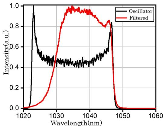
Fig. 3. Comparison of the transmission spectra after the BPF and the oscillator.
