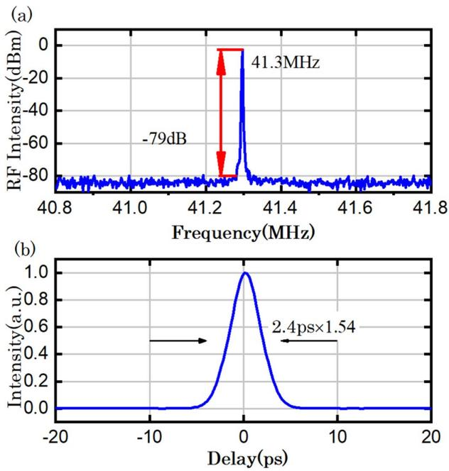
Fig. 2. (a) RF spectrum of the oscillator. (b) The AC trace of the laser pulses from the oscillator.
