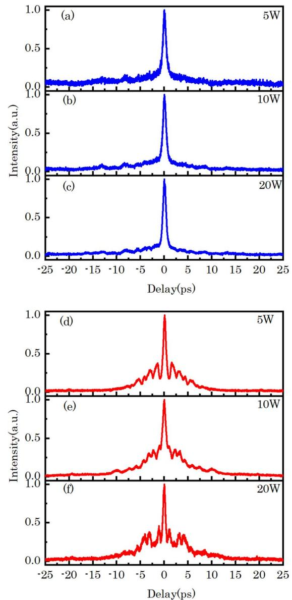
Fig. 6. AC traces at different pulse energies (a)–(c) with BPF and (d)–(f) without BPF.
