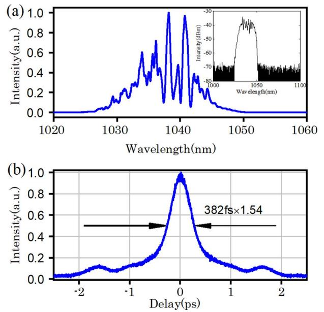
Fig. 4. (a) Spectral distribution from amplified pulses on linear and logarithmic scale; (b) AC trace of compressed pulses.
