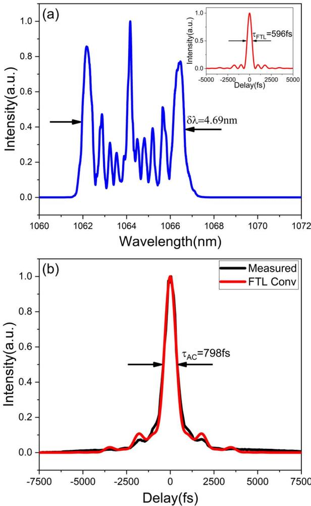
Fig. 3. Characterization of the laser pulses after the compression unit. (a) Spectrum after MPC device; inset: calculated FTL pulse duration. (b) Intensity autocorrelation trace after compressor (black) and convolution of the FTL pulse (red).
