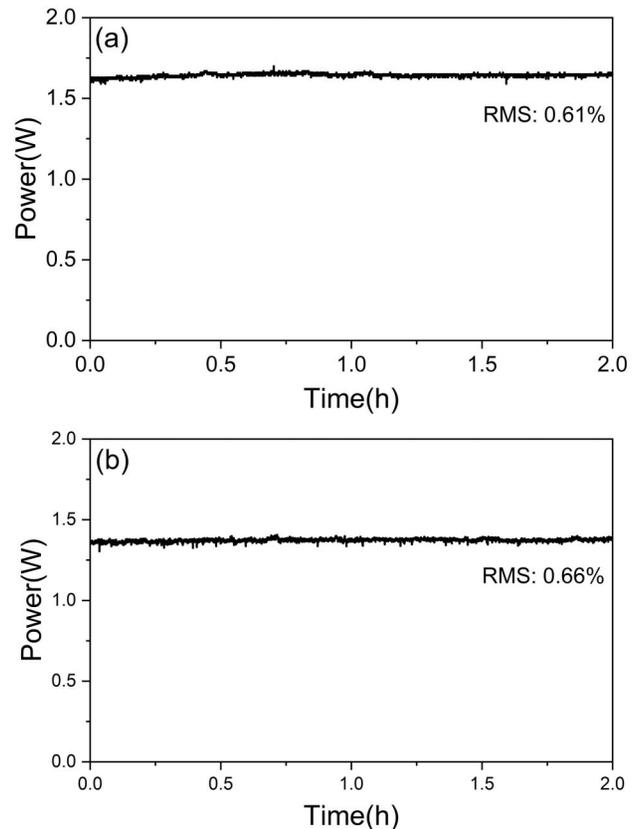
Fig. 4. Long-term power stability of the (a) Nd:YVO<sub>4</sub> picosecond laser and (b) MPC.
