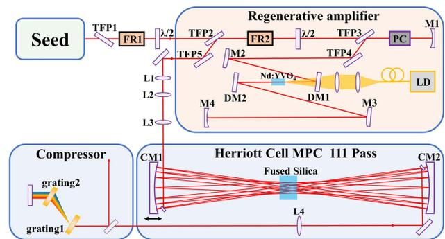
Fig. 1. Experimental setup: Nd:YVO<sub>4</sub> regenerative amplifier followed by the MPC and grating compressor. TFP1-TFP5, thin film polarizers; FR1, FR2, Faraday rotators;  $\lambda/2$ , half-wave plate; PC, Pockels cell; M1-M4, regenerative cavity mirrors; DM1, DM2, dichroic mirrors, with high transmission (HT) at 808 nm and HR at 1064 nm; LD, laser diode at 808 nm; L1-L4, lenses; CM1, CM2, concave mirrors.
