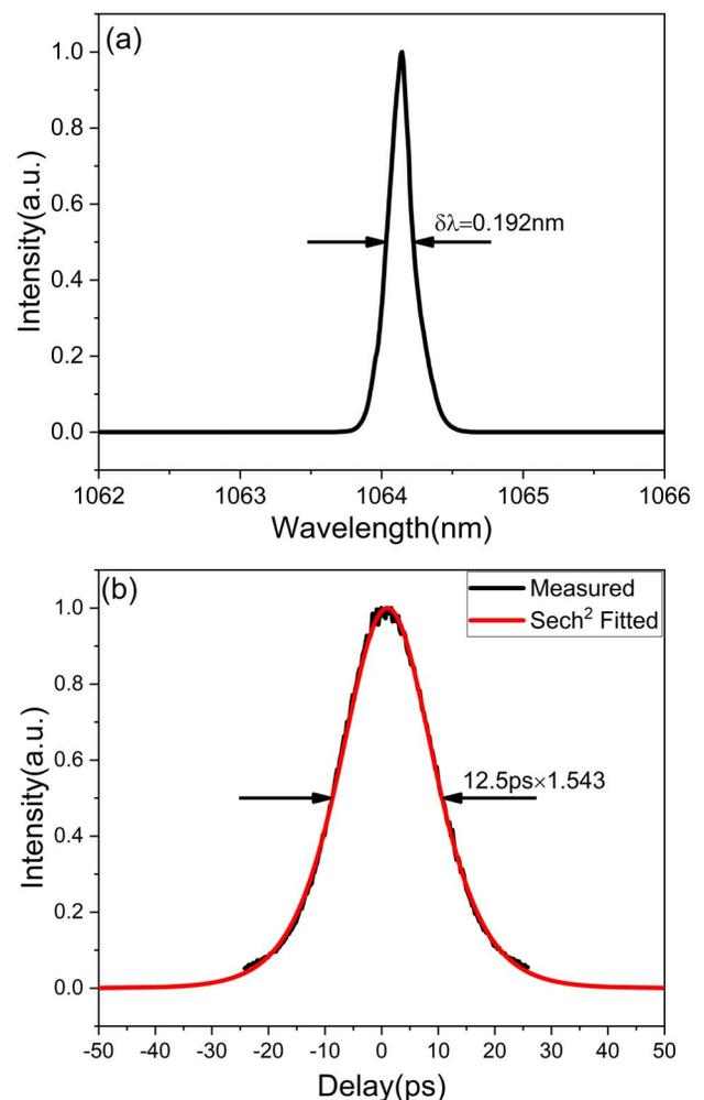
Fig. 2. Characterization of the Nd:YVO<sub>4</sub> regenerative amplifier. (a) Spectrum and (b) intensity autocorrelation trace.
