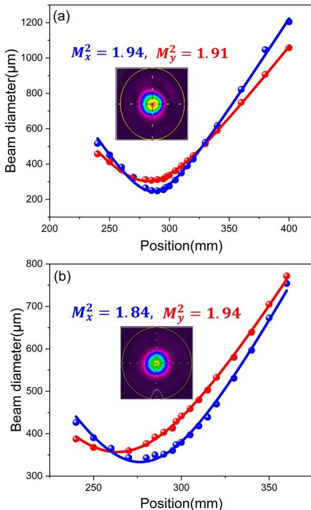
Fig. 5. Beam quality ( $M^2$ ) [a] before and [b] after the MPC device.
