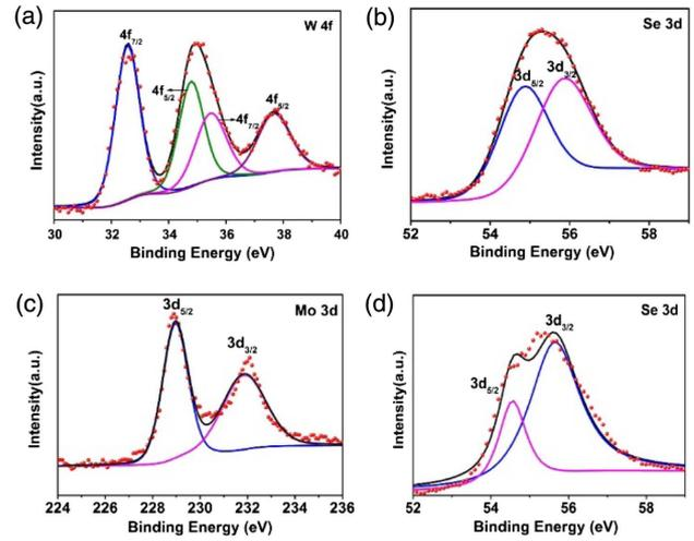
**Fig. 5.** (a) and (b) are the XPS profiles of WSe<sub>2</sub>. (c) and (d) are the XPS profiles of MoSe<sub>2</sub>.
