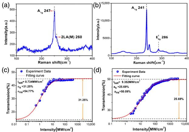
**Fig. 4.** (a) Raman spectrum of the WSe<sub>2</sub> SA. (b) Raman spectrum of the MoSe<sub>2</sub> SA. (c) Non-linear saturable absorption of the WSe<sub>2</sub> SA. (d) Non-linear saturable absorption of the MoSe<sub>2</sub> SA.
