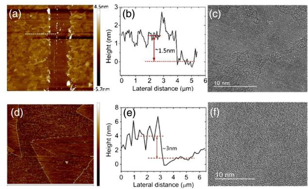
**Fig. 1.** (a) AFM overview of  $\text{WSe}_2$ . (b) Function curve of height and lateral distance of the  $\text{WSe}_2$  SA. (c) TEM detail image of the  $\text{WSe}_2$  SA at scale bar length of 10 nm. (d) AFM image of  $\text{MoSe}_2$ . (e) Function curve of height and lateral distance of the  $\text{MoSe}_2$  SA. (f) TEM detail image of the  $\text{MoSe}_2$  SA at high resolution of 10 nm.
