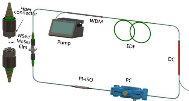
**Fig. 6.** Schematic diagram of the passively  $Q$ -switched pulse fiber laser on the basis of  $WSe_2$  and  $MoSe_2$  SAs. Pump is the laser diode with a center wavelength of 976 nm; WDM is the wavelength division multiplexer;  $WSe_2/MoSe_2$  SA is the saturable absorber; EDF is the erbium-doped gain fiber; PI-ISO is the polarization independent isolator; PC is the polarization controller; OC is the optical coupler.
