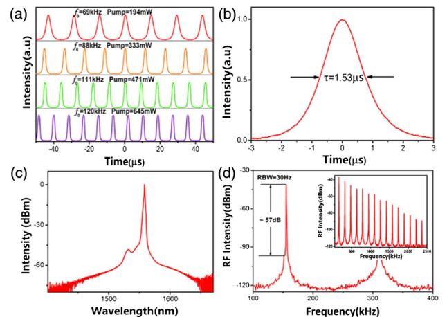
**Fig. 9.** Experimental results of  $Q$ -switched fiber laser based on the  $MoSe_2$  SA. (a) Pulse trains at different power levels. (b) Single pulse sequence at maximum pump power of 680 mW. (c) Optical spectrum. (d) RF spectrum.
