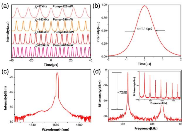
**Fig. 7.** Experimental results of passively  $Q$ -switched pulse fiber laser based on the  $WSe_2$  SA. (a) Pulse trains at different power levels. (b) Single pulse sequence at maximum pump power of 680 mW. (c) Optical spectrum. (d) RF spectrum at 300 Hz RBW.
