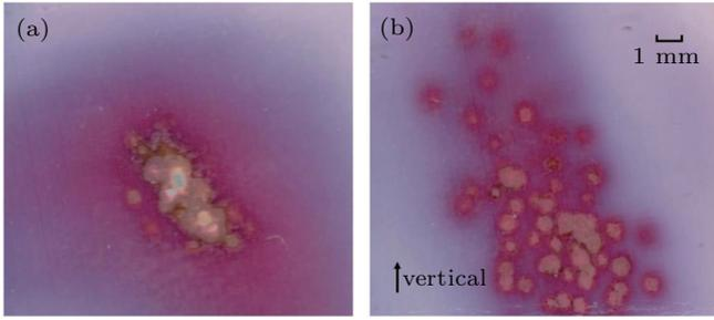
**Fig. 4.** (color online) Marks on photo papers burned by 10-s irradiation (100 shots) of laser pulse at (a) 23-m and (b) 53-m distances.
