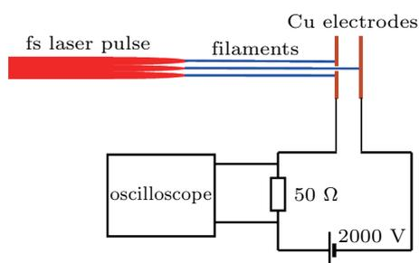
Fig. 2. (color online) Setup of electron density measurement.
