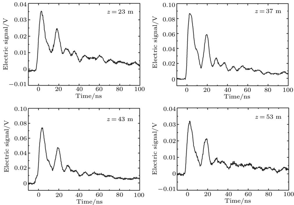
**Fig. 5.** The strongest electric signals of filament at different propagation distances.
