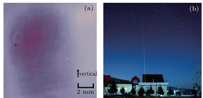
**Fig. 1.** (color online) (a) Initial beam pattern of the TW fs pulse, and (b) long distance filamentation of TW fs laser pulse in atmosphere.
