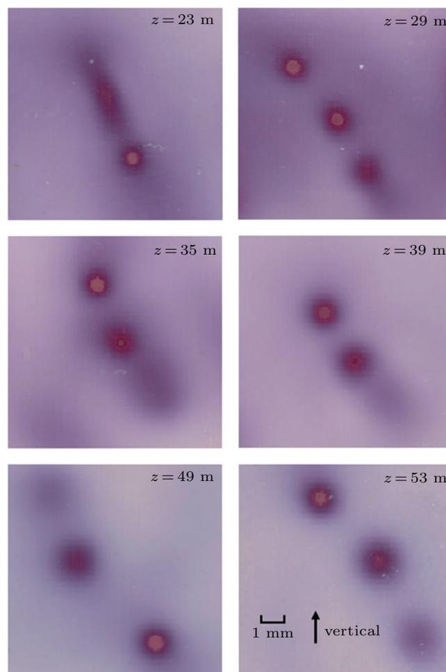
Fig. 3. (color online) Filament structure of laser beam at different propagation distances.
