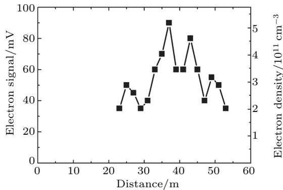
Fig. 6. Peak electric signal (left vertical axis) and electron density (right vertical axis) of filament versus propagation distance.
