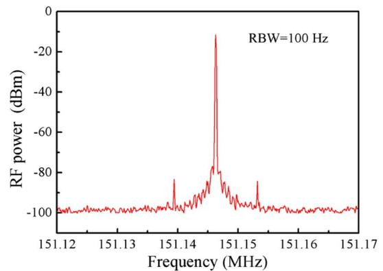
**Fig. 4.** Radio frequency spectrum of the mode-locked Ti:sapphire laser with RBW of 100 Hz.
