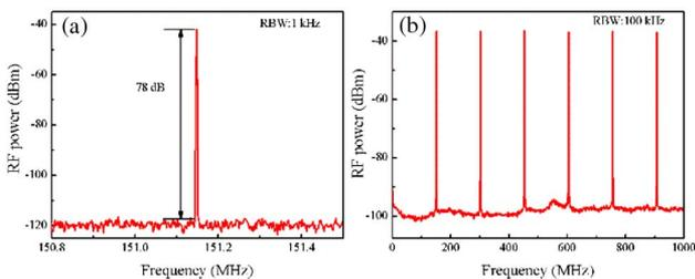
**Fig. 3.** Typical radio frequency spectrum of the Ti:sapphire laser. (a) RF spectrum of the fundamental beat note with the RBW of 1 kHz; (b) wide spectrum of 1 GHz with the RBW of 100 kHz.
