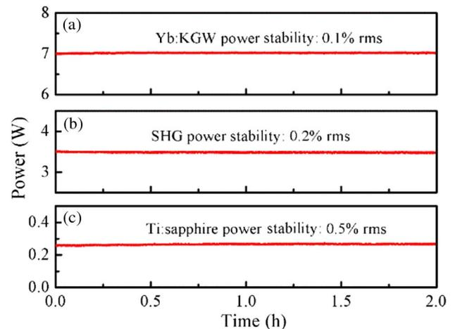
**Fig. 7.** Power stability of the output power in 2 h. (a) Yb:KGW laser; (b) SHG; (c) Ti:sapphire laser.
