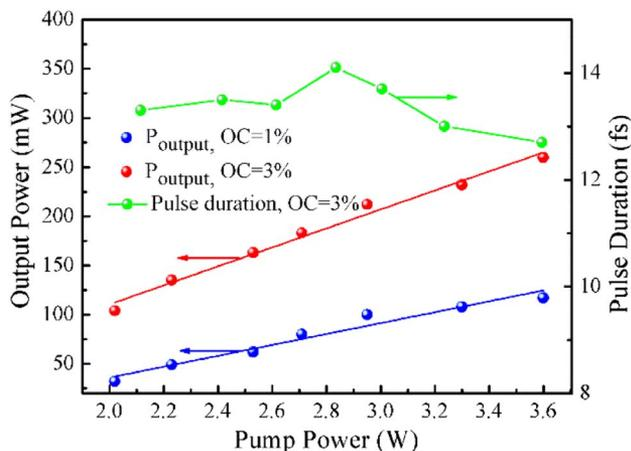
**Fig. 6.** Mode-locked output powers and pulses duration of Ti:sapphire as a function of the pump power.
