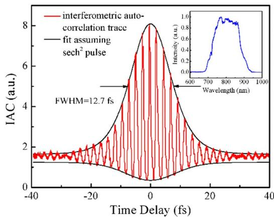
**Fig. 5.** Interferometric autocorrelation traces of the compressed 12.7 fs mode-locked pulse (red curve) with a  $\text{sech}^2$  fitting (black curve) under 3% transmissions. Inset: corresponding the spectrum centered at wavelength of 811 nm.
