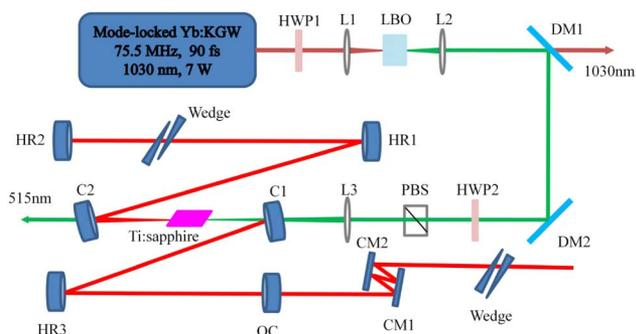
**Fig. 1.** Schematic of the experimental setup for Ti:sapphire laser. L1–L3, lenses with  $f_1 = 100$  mm,  $f_2 = 150$  mm,  $f_3 = 75$  mm; HWP, half-wavelength plate; PBS, polarizing beam splitter; DM1–DM2, dichroic mirrors; C1–C2, concave spherical mirrors with  $R = 100$  mm; HR1–HR3, plane mirrors; OC, 3% output coupler; CM1–CM2, chirped mirrors.
