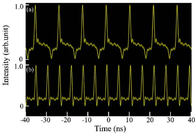
**Fig. 2.** Mode-locked pulse trains at 10 ns/div: (a) mode-locked Yb:KGW laser; (b) mode-locked Ti:sapphire laser.
