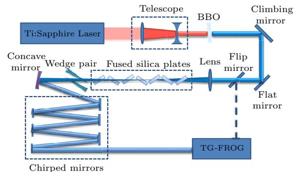
**Fig. 1.** The experimental setup for 400 nm continuum generation and compression.
