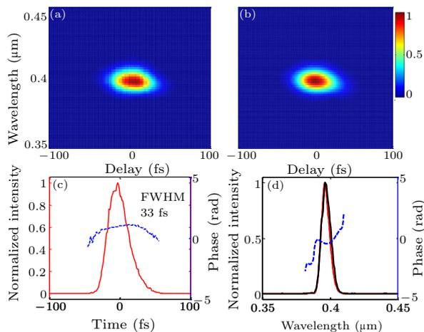
**Fig. 2.** Characterization of  $33 \text{ fs}$  pulse before thin solid plates. (a) The experimental FROG trace, (b) the retrieved FROG trace, (c) the retrieved pulse shape (red solid line) and the retrieved phase (blue dashed line), and (d) the measured spectrum (black solid line), the retrieved spectrum (red solid line) and the retrieved phase (blue dashed line).
