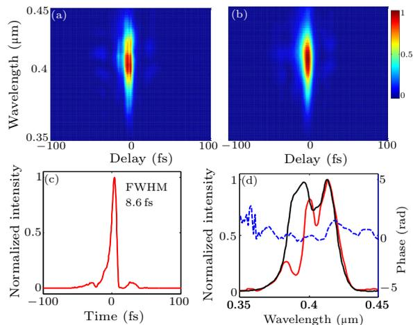
**Fig. 4.** The compressed  $8.6 \text{ fs}$  pulse characterized by TG-FROG, (a) the experimental FROG trace, (b) the retrieved FROG trace, (c) the retrieved pulse shape (red solid line), and (d) the measured spectrum (black solid line), the retrieved spectrum (red solid line) and the retrieved phase (blue dashed line).
