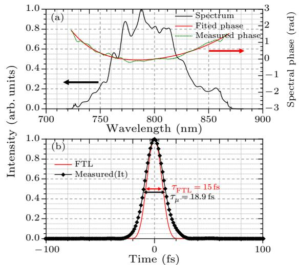
**Fig. 6.** Spectral and temporal properties of the amplified XPW pulses. (a) Black curve: measured spectrum; red curve: fitted spectral phase; and green curve: measured phase. (b) Black dots: measurement of the pulse duration. Red line: FTL calculated from the spectrum.
