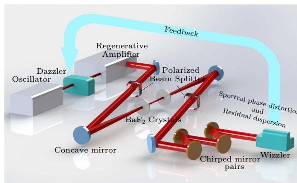
**Fig. 1.** Detailed structure design of the cascaded XPW filter.
