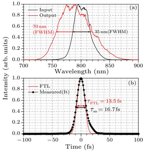
**Fig. 4.** Spectral and temporal properties of XPW pulses. (a) Black curve: measurement of the spectrum at the regenerative amplifier (compressed), with the FWHM of 35 nm. Red curve: measurement of the spectrum after the XPW, with the FWHM of 70 nm. (b) Black dot: measurement of the pulse duration of the compressed XPW output. Red line: FTL pulse duration calculated from the spectrum.
