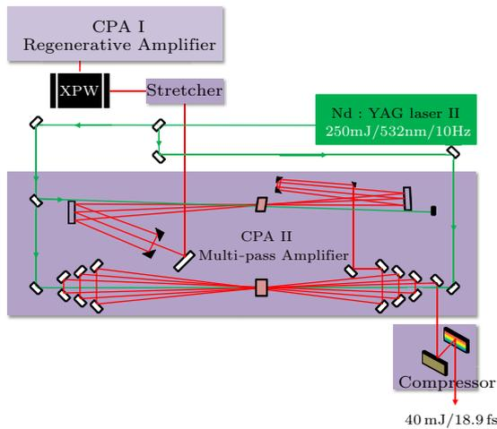
**Fig. 5.** Schematic diagram of XPW built in the double-CPA system with the peak-power of 2 TW.
