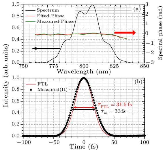
**Fig. 2.** Spectral and temporal properties of the XPW driving pulses. (a) Black curve: measured spectrum; red curve: fitted spectral phase; and green curve: measured spectral phase. (b) Black dot: measurement of the pulse duration before the XPW; and red line: FTL pulse duration calculated from the spectrum.
