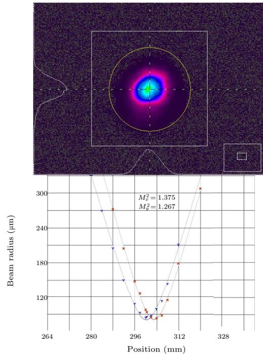
**Fig. 3.** The  $M^2$  factor measurement result of the regenerative amplifier (compressed).
