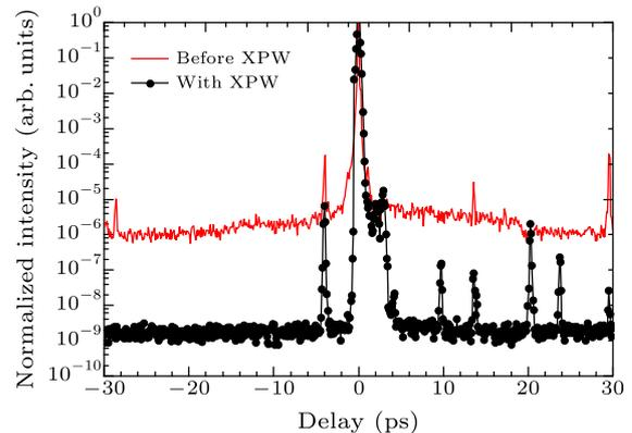
**Fig. 7.** Third-order cross-correlation measurement of the pulses before XPW (red line) and the TW system output pulses after XPW (black dotted line).
