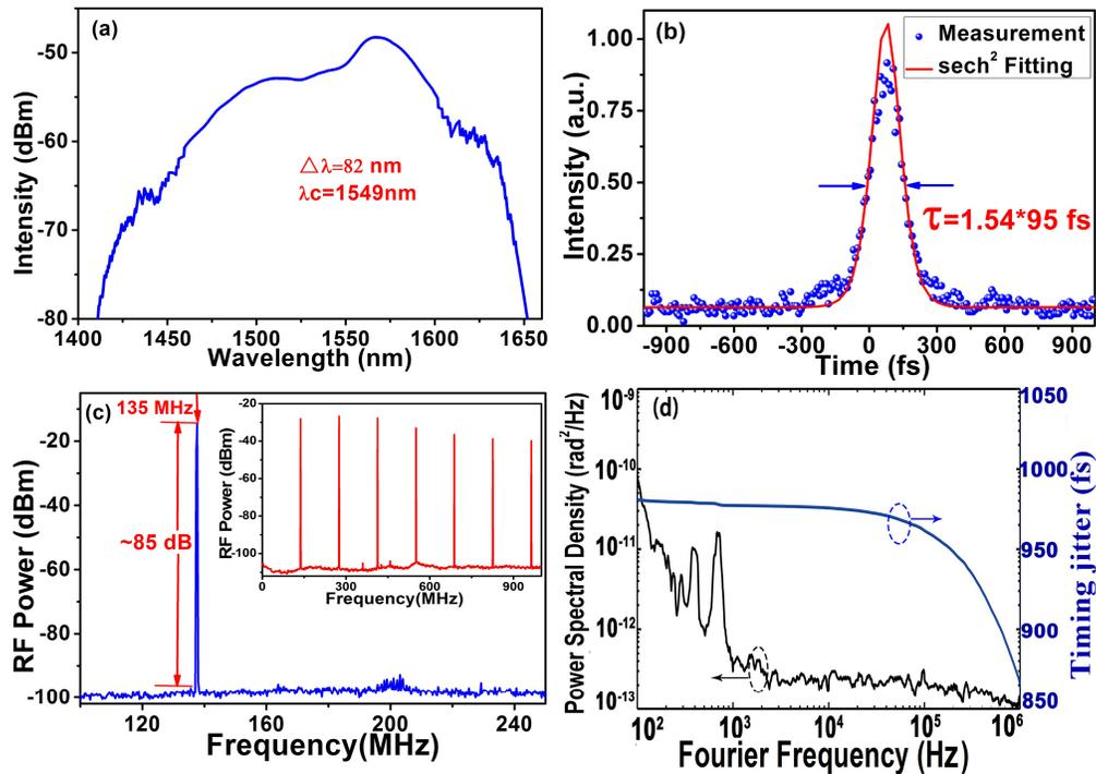
Fig. 6. Experimental results of the passively mode-locked EDF laser with the SMF in the same length. The difference with Fig. 4 is that the fiber-taper WS<sub>2</sub> SA is replaced with the SMF. (a) The 3 dB spectral width is 82 nm at 1549 nm. (b) Intensity autocorrelation trace with 95 fs pulse duration. (c) RF spectrum with 85 dB SNR measured with 10 kHz RBW. (d) Phase noise measurement at 135 MHz, and the timing jitter is about 0.95 ps.
