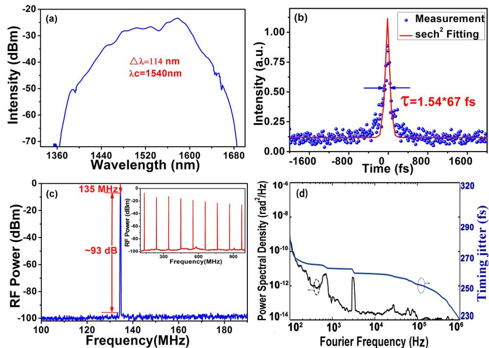
Fig. 5. Experimental results of the passively mode-locked EDF laser with the fiber-taper WS<sub>2</sub> SA. (a) Optical spectrum of the generated pulses. The 3 dB spectral width is 114 nm at 1540 nm. (b) Intensity autocorrelation trace with 67 fs pulse duration. (c) Radio frequency (RF) spectrum with 93 dB SNR measured with 10 kHz RBW. (d) Phase noise measurement at 135 MHz, and the timing jitter is about 290 fs.
