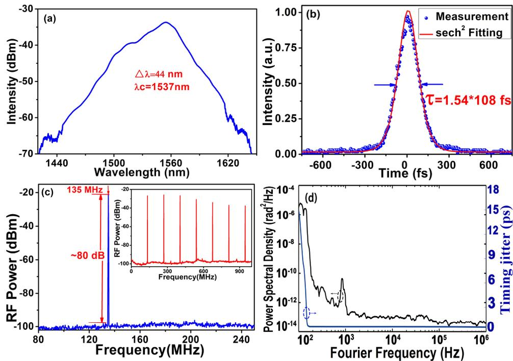
Fig. 7. Experimental results of the passively mode-locked EDF laser with the tapered fiber. The difference with Fig. 4 is that the fiber-taper  $\text{WS}_2$  SA is replaced with the tapered fiber. (a) The 3 dB spectral width is 44 nm at 1537 nm. (b) Intensity autocorrelation trace with 108 fs pulse duration. (c) RF spectrum with 80 dB SNR measured with 10 kHz RBW. (d) Phase noise measurement at 135 MHz, and the timing jitter is about 15 ps.
