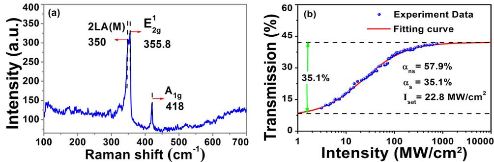
Fig. 2. (a) Raman spectrum of the WS<sub>2</sub> on the fiber-taper SA. Two optical phonon modes are at 355.8  $\text{cm}^{-1}$  and 418  $\text{cm}^{-1}$ , respectively. The typical longitudinal acoustic mode is at 350  $\text{cm}^{-1}$ . (b) Nonlinear saturable absorption of the WS<sub>2</sub> SA. The modulation depth is 35.1%, the saturation intensity is 19.8  $\text{MW}/\text{cm}^2$ , and the non-saturable loss is 59.5%.
