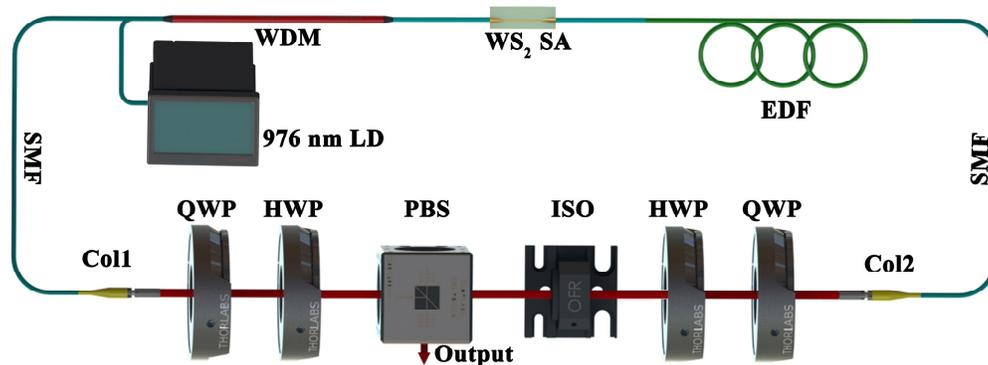
Fig. 4. Configuration of the passively mode-locked EDF laser with the fiber-taper WS<sub>2</sub> SA. LD is the laser diode, WDM is the wavelength-division multiplexer, SMF is the signal mode fiber, Col. is the collimator, QWP is the quarter wave plate, HWP is the half wave plate, PBS is the polarization beam splitter, ISO is the polarization-dependent isolator, and EDF is the erbium-doped fiber.
