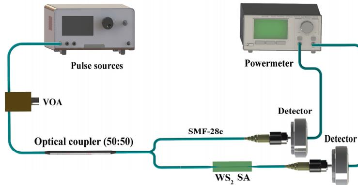
Fig. 3. Standard two-arm transmission setup.
