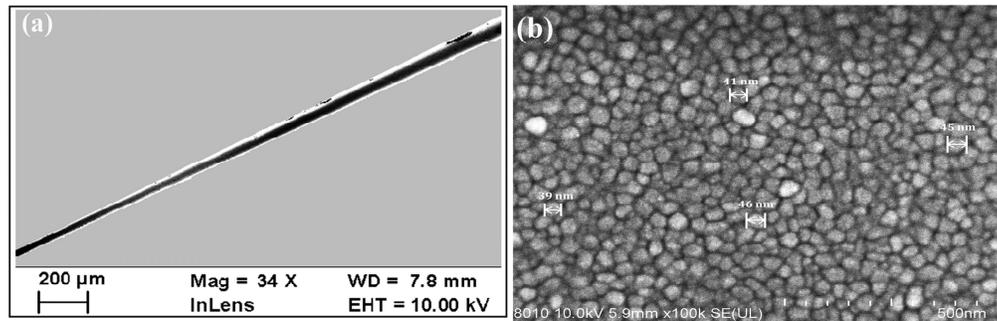
Fig. 1. (a) The SEM image for the taper waist of the WS<sub>2</sub> SA. The waist diameter is 12  $\mu\text{m}$ , and the effective length of the fused zone is 3 mm. (b) Film surface of the WS<sub>2</sub> SA.
