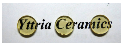
Fig. 1. (color online) Photo of the Yb–Ho: (YLa) 2 O 3 transparent ceramic (3 mm thick).
