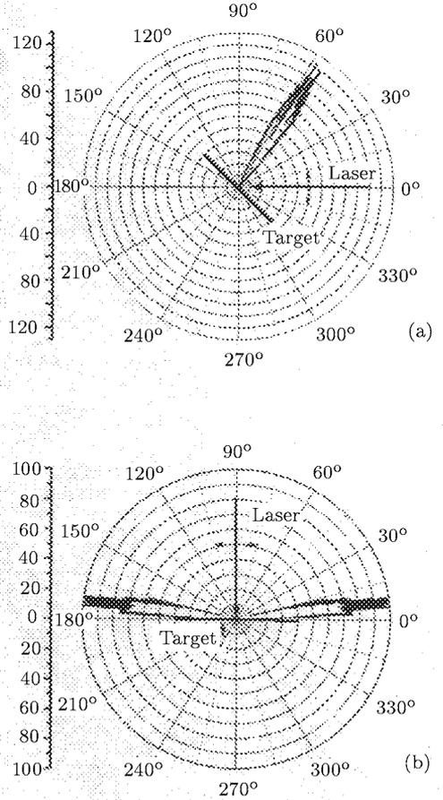
Fig. 3. Cutaway view of angular distribution of hot electrons generated from a solid target irradiated by (a) p-polarized laser pulses and (b) s-polarized laser pulses.
