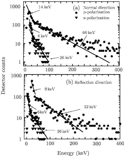
Fig. 2. Detector counts for  $\gamma$ -ray photons versus photon energy.
