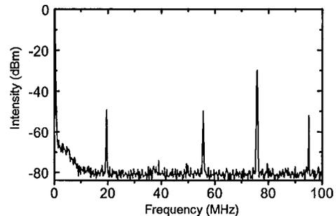
Fig. 3. Frequency spectrum obtained by heterodyning of the SH of the Ti:sapphire laser with the TH of Cr:forsterite lasers.
