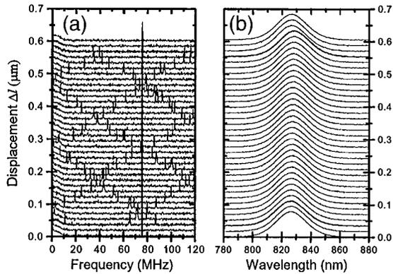
Fig. 4. (a) Beat signals acquired by shifting of the mirror displacement and (b) corresponding spectra of the Ti:sapphire laser.
