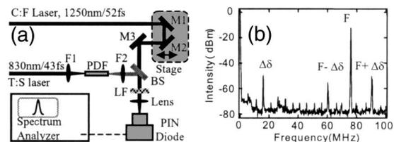
Fig. 1. (a) Experimental setup for heterodyning the Cr:forsterite (C:F) laser with the continuum from the Ti:sapphire (T:S) laser: PDF, 25-cm PCF with a 1.8- $\mu\text{m}$  core diameter; F1, F2, 40 $\times$  objective lenses; BS, metal beam splitter; LF, optical filter. M1–M3, gold mirrors. (b) Observed beat signal.
