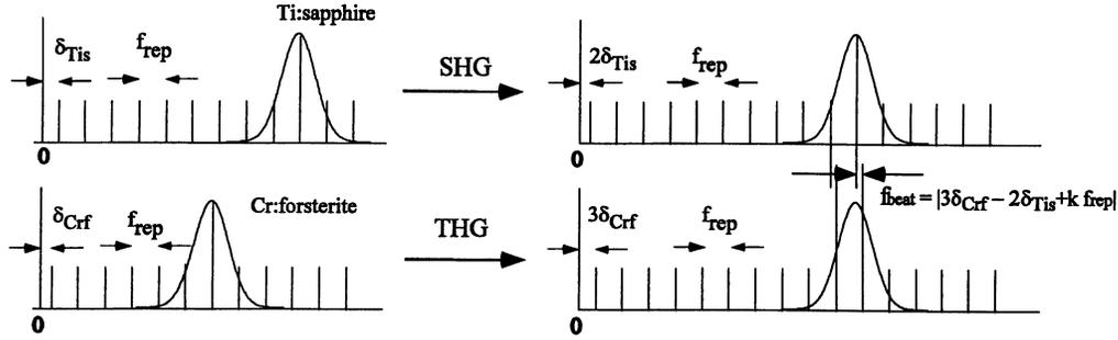
Fig. 1. Schematic of CEO frequency-relation measurement in a dual-wavelength laser in the frequency domain. Comb spacings ( $f_{\text{rep}}$ ) are the same because the Ti:sapphire laser and Cr:forsterite laser are passively synchronized. Spectra of the frequency-doubled Ti:sapphire and the frequency-tripled Cr:forsterite laser overlap at 415 nm, and a beat signal can be observed. SHG is second-harmonic generation and THG third-harmonic generation.
