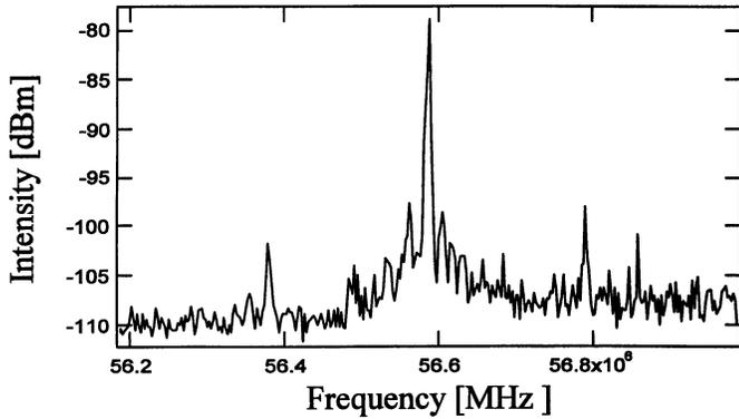
Fig. 4. Locked beat signal obtained by a spectrum analyzer with an average of ten traces. Beat frequency is locked to three-fourths of the repetition rate. Span is 1 MHz with an RBW of 3 kHz, and observed spectrum width is also the RBW.
