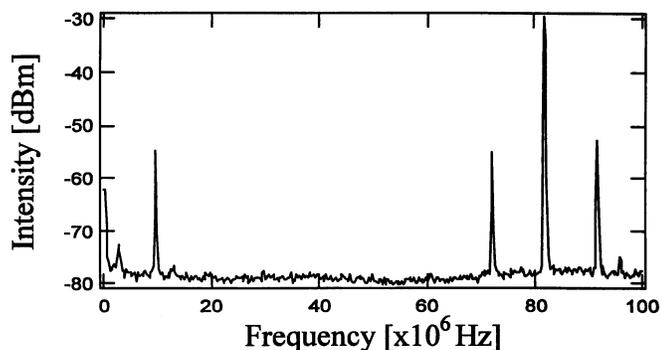
Fig. 8. Locked beat spectrum measured by a spectrum analyzer in 100-MHz span. Over 100 traces are averaged. RBW is 100 kHz and locked spectrum width is also RBW.
