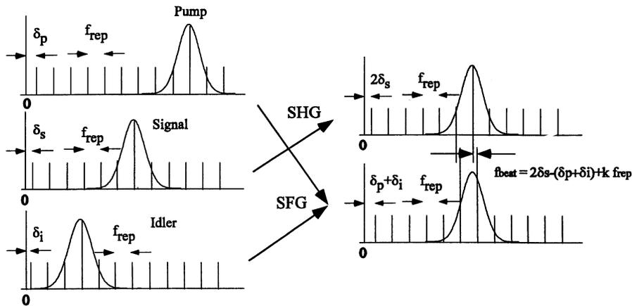
Fig. 5. Schematic of the CEO-frequency relation measurement in subharmonic OPO in the frequency domain. Optical frequencies of the doubled signal and the sum frequency between the pump and the idler overlap. Beat signal can thus be obtained by superposing them. SFG is sum-frequency generation and SHG, second-harmonic generation.
