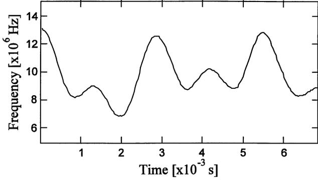
Fig. 3. Beat signal dynamics in free-running operation measured by a digital spectrum analyzer. Horizontal axis represents time, and the vertical axis, frequency. Frequency and time spans are 10 MHz and 6.8 ms. Beat frequency moves more than 5 MHz within 1 ms.
