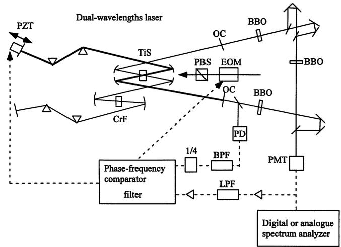
Fig. 2. Experimental setup for CEO frequency-relation control in a dual-wavelength laser. Solid lines indicate the optical paths, and dashed lines represent the electronic paths. Bold lines show the optical paths in the Ti:sapphire laser cavity. TiS, Ti:sapphire crystal; CrF, Cr:forsterite crystal; OC, output coupler; PBS, polarized beam splitter; PD, photo diode; PMT, photo-multiplier tube; LPF, low-pass filter; "1/4", frequency divider.
