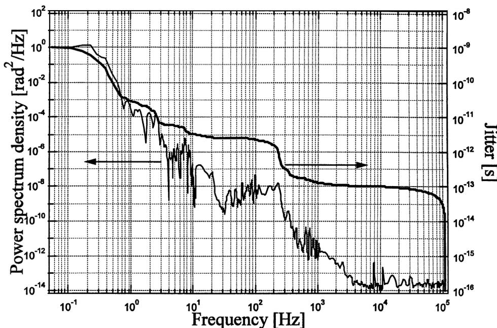
Fig. 7. Power spectrum density and calculated timing jitter of the Ti:sapphire laser without control.
