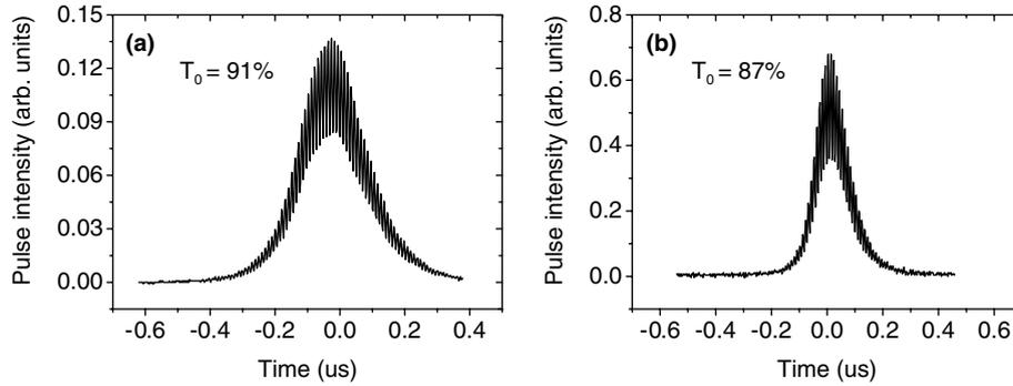
Fig. 2. Temporal profiles of the Q-switched and mode-locked laser pulses using different  $T_0$  of the saturable absorbers when the incident pump power was 5 W.
