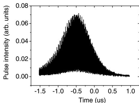
Fig. 5. Temporal profile of the Q-switched and mode-locked laser pulses when the cavity length was 72.6 cm.
