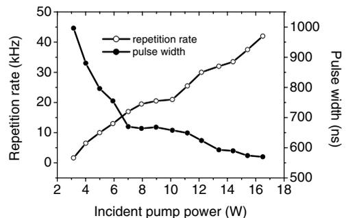
Fig. 4. The repetition rate and pulse width of the Q-switched envelope as a function of the incident pump power.
