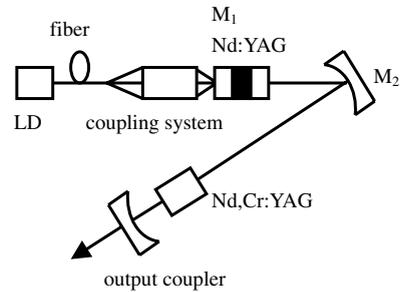
Fig. 1. Schematic of a passive Q-switched and mode-locked 946 nm Nd:YAG laser.
