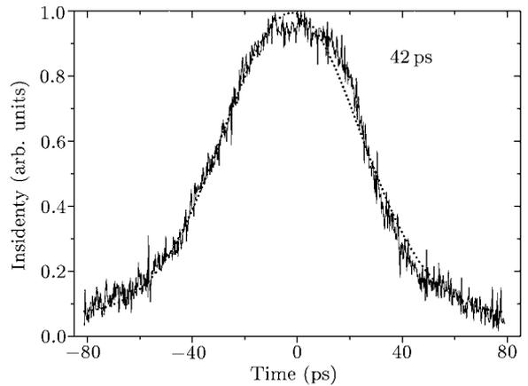
**Fig. 5.** The measured profile of autocorrelation trace, corresponding to the pulse width of 42 ps, and the dotted line shows the Gaussian assumption.
