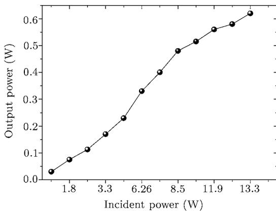
**Fig. 3.** Dependence of the mode-locked average output versus incident power for the laser.
