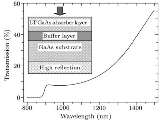
**Fig. 1.** Measured transmission spectrum of the LTGAM. The inset shows the schematic structure of the LTGAM, and the incident laser is vertical to the LT GaAs absorber layer, as shown by the arrowhead.
