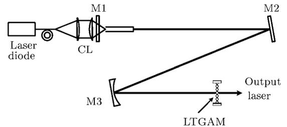
**Fig. 2.** The schematic of the mode-locking laser. CL: the collimating and focusing system; M1: input mirror; M2: folding mirror; M3: focusing mirror; LTGAM: low temperature GaAs mirror (OC = 9%).
