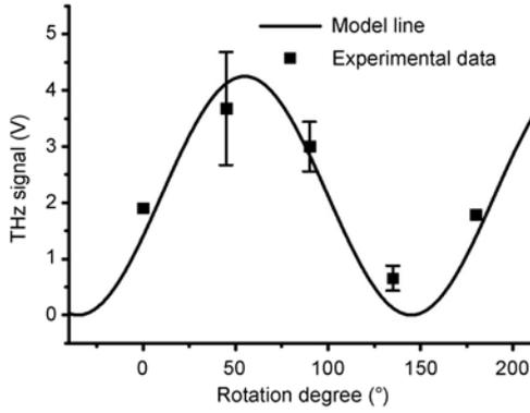
**Figure 2** THz signal measured by the detector (squares) and the fitting line induced by the transient current model (line).
