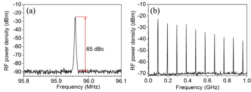
**Figure 3.** (a) RF spectrum at the fundamental beat note. (b) RF spectrum of 1 GHz wide-span range.
