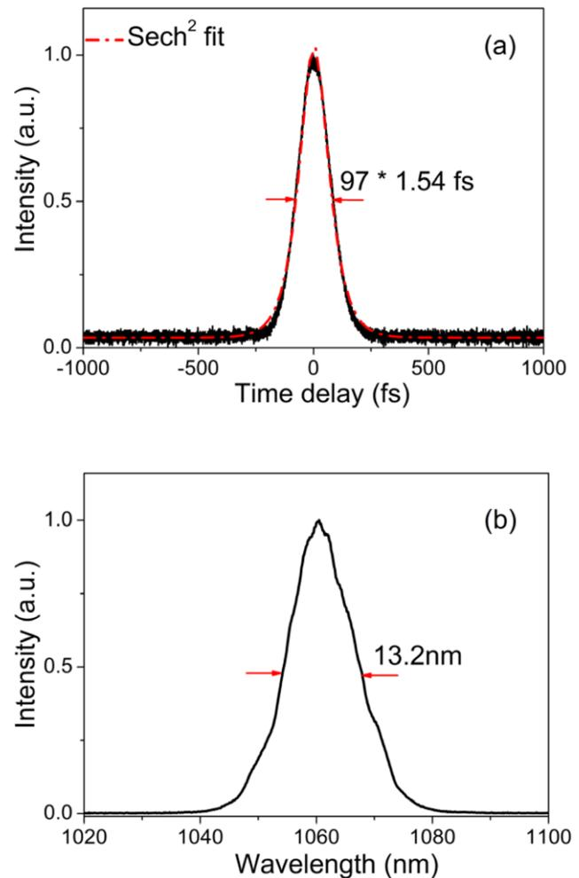
**Figure 2.** (a) Intensity autocorrelation trace and (b) laser spectrum of the mode-locking operation with 0.3% OC. The output power was 102 mW under 925 mW pump power.
