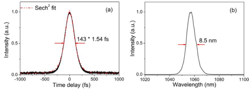
**Figure 4.** (a) Intensity autocorrelation trace of 143 fs pulses and (b) the corresponding laser spectrum with the 1.6% OC. The output power was 232 mW.
