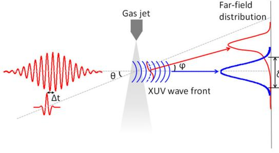
FIG. 1. Principle illustration of the scheme of the IAP generation. A long driving pulse and a short gating pulse with a noncollinear angle  $\theta$  and time delay  $\Delta t$  overlap in the gas medium. The distorted XUV wave front induced by the gating pulse in the overlapping region lead to off-axis IAP with a propagation angle  $\varphi$ .
