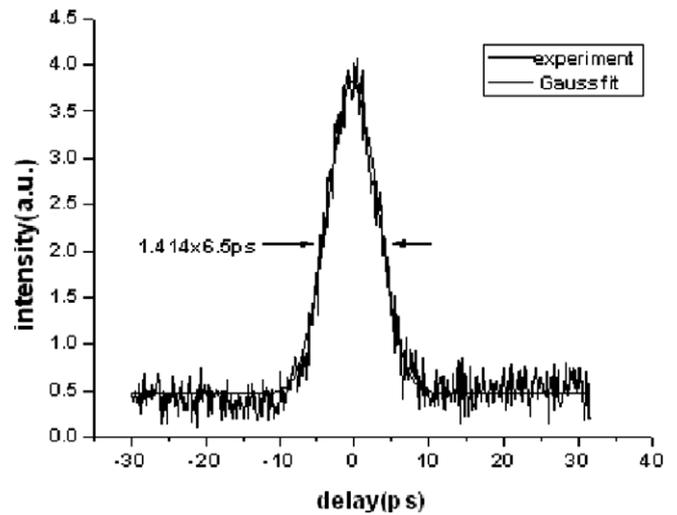
**Fig. 4.** The measured autocorrelation trace of the pulses.
