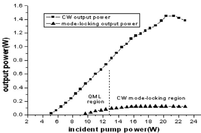
**Fig. 2.** Dependence of the laser CW output and mode-locking output on the incident pump power. ■ and ▲ indicate the CW output power and mode-locking output power, respectively. QML: Q-switched mode-locking.
