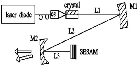
**Fig. 1.** Experimental layout of passively mode-locked Nd:GdVO<sub>4</sub> laser. M1: HR at 912 nm, radius of curvature (RoC) is 300 mm; M2:  $r = 1\%$  at 912 nm, radius of curvature (RoC) is 100 mm; CS: coupling system; L1: 260 mm, L2: 500 mm, L3: 67 mm.
