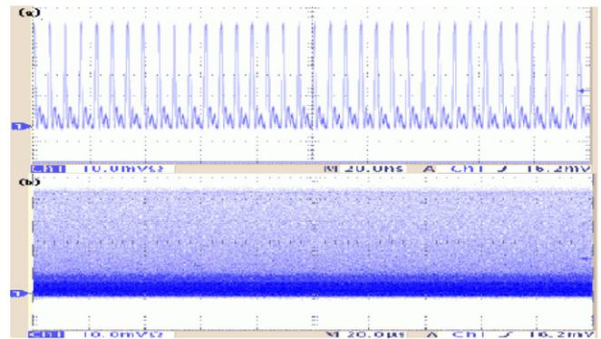
**Fig. 3.** Pulse trains observed with two different time scales: (a) 20 ns and (b) 20 us.
