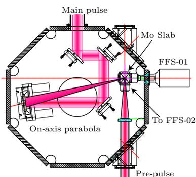
**Fig. 1.** A diagram of the basic experimental setup. A crossed slit camera was installed at the top-front of the target. Another flat field spectrometer with space imaging ability was used to measure the self emission of the plasma medium. Neither of the latter two instruments is shown on the diagram.
