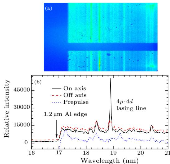
**Fig. 2.** (a) A time integrated image from the flat field spectrometer on the axis. The  $4d - 4p$  Ni-like Mo lasing line at 18.9 nm is clearly seen. (b) A spatially integrated spectrum near the 18.9 nm lasing line (solid line). A plot of the spectra of the off-axis emission (dashed line) when lasing and a plot of the spectra with only pre-pulse launched (dotted line) are also shown.
