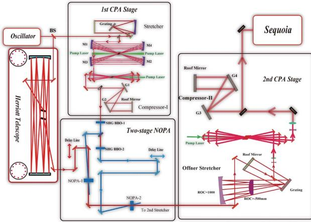
Fig. 1. (Color online) Schematic experimental setup of the femtosecond NOPA.
