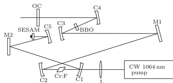
**Fig. 1.** Schematic diagram of the experimental setup. L: lens with focal length of 100 mm; C1-C5: concave mirrors with ROC of 100 mm.
