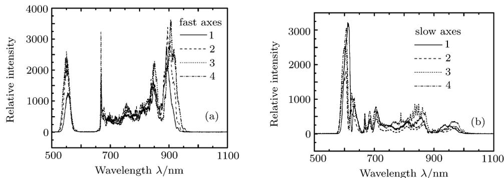
**Fig.5.** Spectrum of radiation at the output of the 5-cm length PCF measured for an input power of 320 mW, and 10-fs 823-nm pump pulses polarized along (a) the fast and (b) the slow axes of the fibre core. The curves 1, 2, 3, and 4 in the figure indicate the four results of the repeated measurement.
