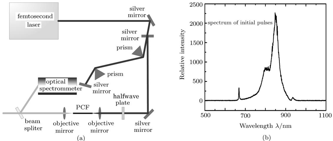
**Fig.2.** (a) Diagram of the experimental setup. (b) Spectrum of initial pulses.
