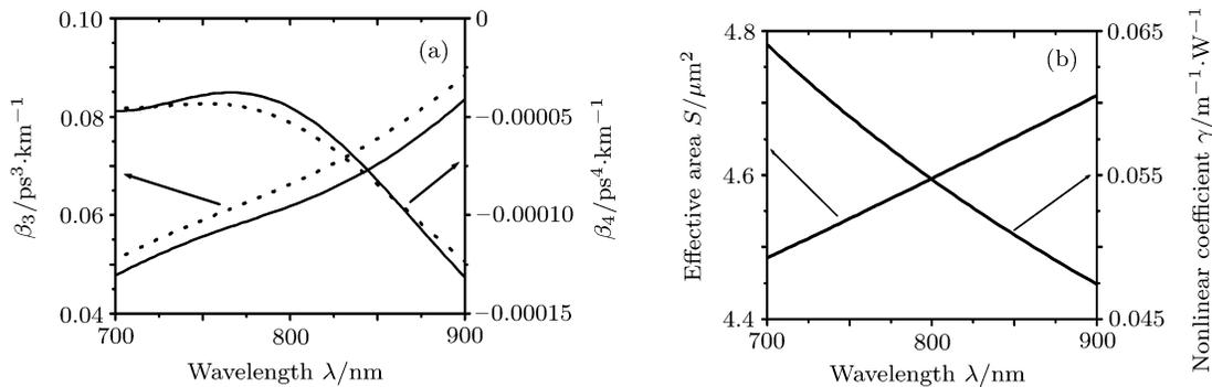
**Fig.4.** (a) The high-order dispersion  $\beta_3$  and  $\beta_4$  corresponding to the slow (solid lines) and fast (dotted lines) fundamental modes as a function of wavelength  $\lambda$ . (b) The effective area  $S$  and nonlinear coefficient  $\gamma$  corresponding to the fundamental mode as a function of wavelength  $\lambda$ , in which lines corresponding to the slow and fast fundamental modes are superposed.
