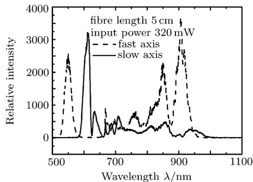
**Fig.6.** The comparison between output spectra at the PCF corresponding to pump pulses polarized along the slow and the fast axes of the fibre core.
