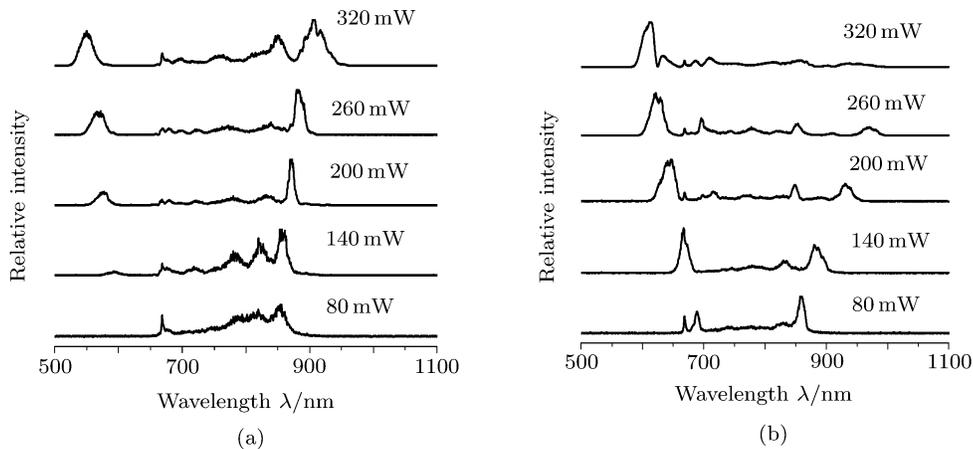
**Fig.3.** The spectra of radiation at the output of the 5-cm length PCF measured for different input powers of 10-fs 823-nm pump pulses polarized along (a) the fast and (b) the slow axes of the fibre core. The average input power is 80 mW, 140 mW, 200 mW, 260 mW, and 320 mW, respectively.
