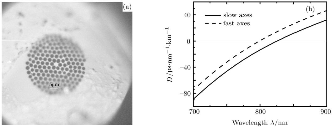
**Fig.1.** (a) A microscopic cross-sectional image of the photonic crystal fibre. (b) Group-velocity dispersion calculated for the slow and fast fundamental modes in an elliptical-core photonic crystal fibre as shown in Fig.1(a).
