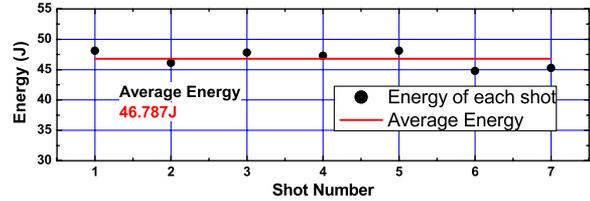
Fig. 2. (Color online) Measured output energies for 105 J pump energy in the booster amplifier. For the seven-shot measurements, the maximum energy was 48.1 J and the minimum energy was 44.8 J. The rms was about 1.5%.
