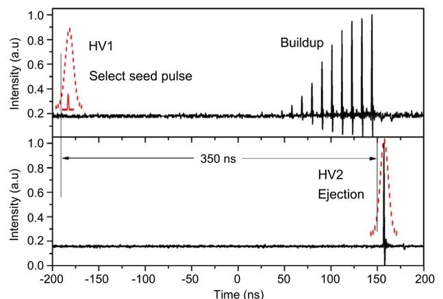
Fig. 3. (Color online) Buildup process of amplification and the dumped amplified pulse from the ring regenerative amplifier. The function principle of double-gating PC is also sketched with a red dashed curve.
