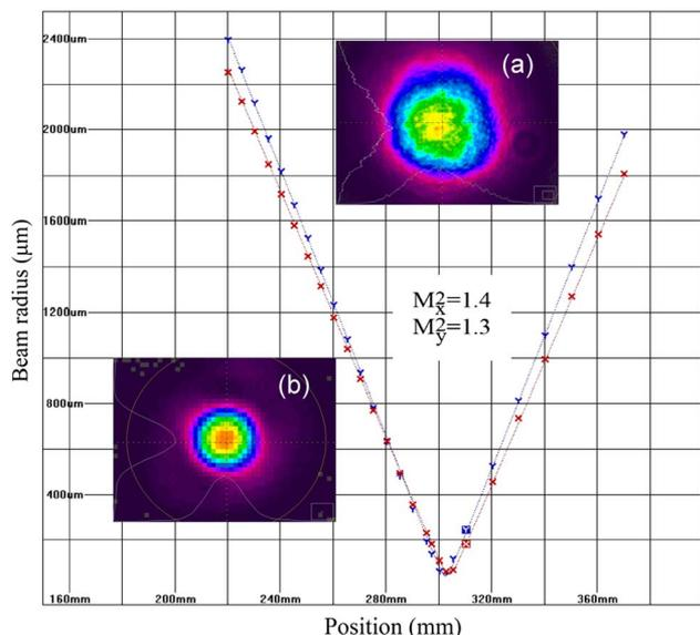
Fig. 8. (Color online) (a) Near-field and (b) far-field beam profiles and M2 factor of the compressed pulse.
