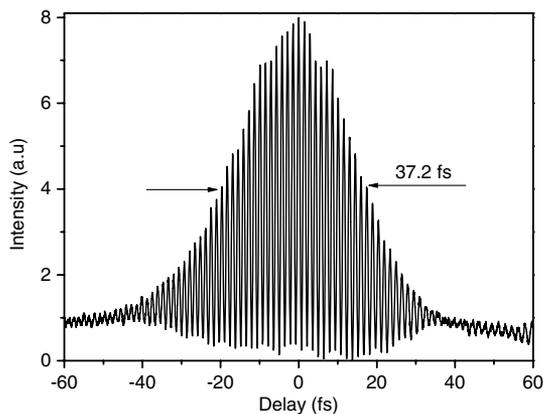
Fig. 5. Interference autocorrelation trace of the pulses after the compressor.
