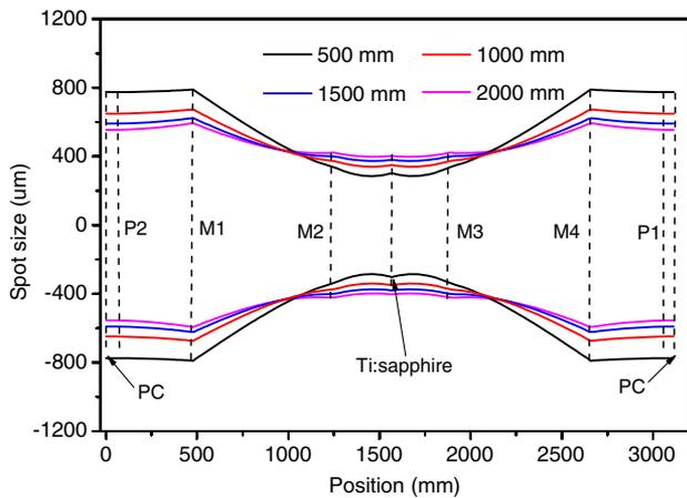
Fig. 2. (Color online) Simulation of spot size in the cavity with different thermal focal length of Ti:sapphire crystal. The straight dashed lines show the internal elements' positions.
