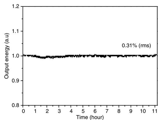
Fig. 7. Energy stability of the pulses after compressor over more than 11 h.
