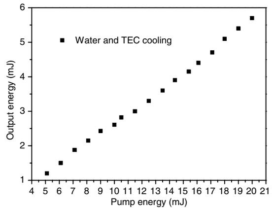
Fig. 6. Output energy extracted from the ring regenerative cavity as a function of pump energy.
