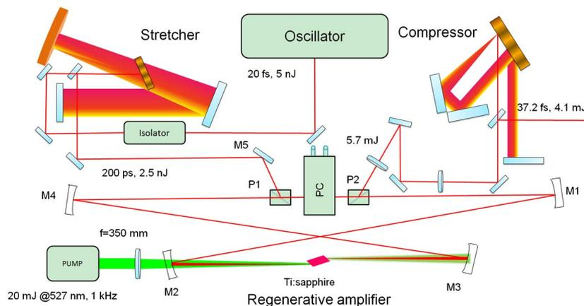
Fig. 1. (Color online) Schematic of the ring regenerative amplifier system, a femtosecond Ti:sapphire laser oscillator, a stretcher, and a compressor are drawn in this figure.
