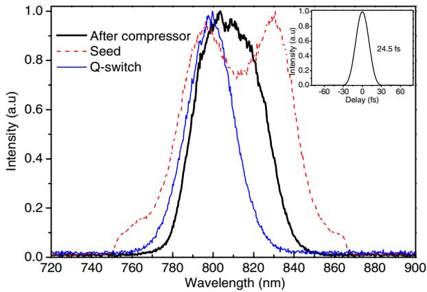
Fig. 4. (Color online) Spectra of seeding laser pulse (dashed curve), *Q*-switched amplified laser pulse (thin curve), and compressed laser pulse (thick curve). The inset shows transform-limited pulse duration of the amplified laser spectrum.
