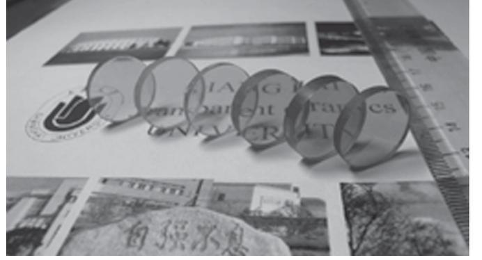
Fig. 1. Photograph of (Nd<sub>x</sub>Y<sub>0.9-x</sub>La<sub>0.1</sub>)<sub>2</sub>O<sub>3</sub> transparent ceramics. From left to right,  $x = 0.005, 0.01, 0.015, 0.02, 0.025,$  and  $0.04$ , respectively.
