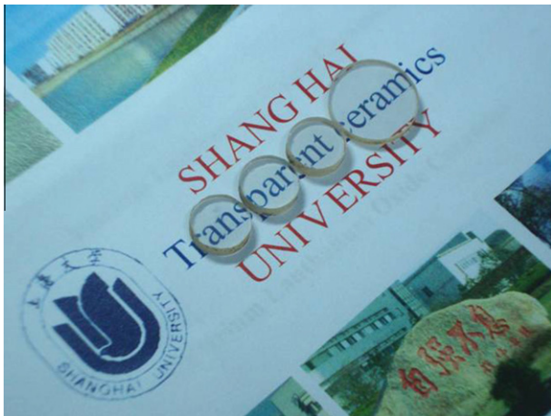
Fig. 1. Photo of Yb:(La 0.10 Y 0.90 ) 2 O 3 transparent ceramic.
