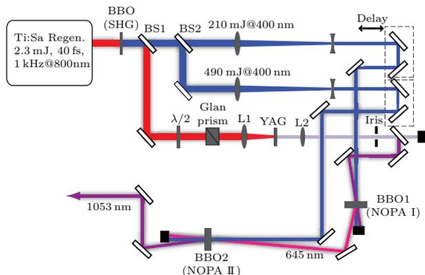
**Fig. 1.** (Color online) The schematic layout of the NOPAs system.
