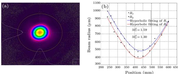
**Fig. 6.** (Color online) Near-field beam profile and  $M^2$  factor of the 1053 nm idler pulse.
