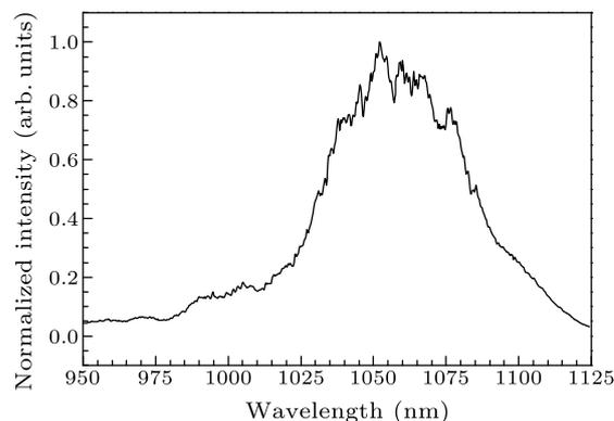
**Fig. 3.** Spectrum of the 1053 nm idler pulse.
