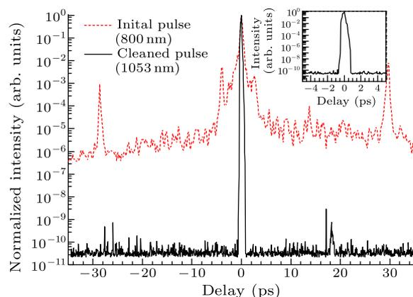
**Fig. 2.** (Color online) Third-order correlation traces of the initial 800 nm pulse (red dashed curve) and the cleaned 1053 nm idler pulse (black solid curve) within the time scale from  $-35$  ps to 35 ps. The inset expands the 1053 nm idler pulse to the time scale of 5 ps before the main pulse.
