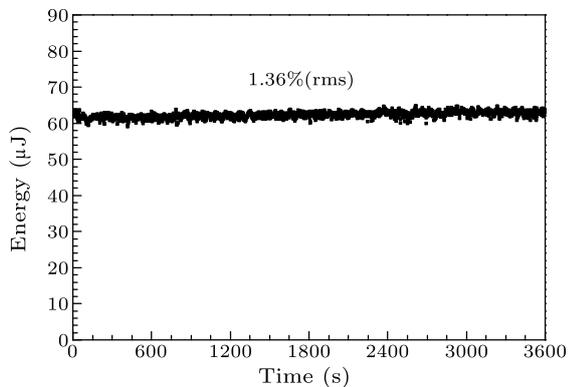
**Fig. 5.** Energy stability of the 1053 nm idler pulse within one hour.
