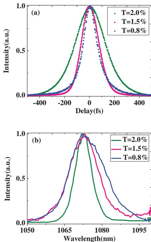
**Figure 3.** (a) Autocorrelation traces of the Kerr-lens mode-locked pulses under three different transmissions ( $T = 0.8\%$ ,  $1.5\%$  and  $2.0\%$ , respectively). (b) The corresponding spectra of the Kerr-lens mode-locked pulses under three different transmissions ( $T = 0.8\%$ ,  $1.5\%$  and  $2.0\%$ , respectively).
