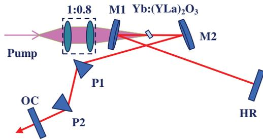
**Figure 1.** Schematic of the experimental setup. M1 and M2: curved high reflection mirrors with ROC=75 mm; HR: high reflection plane mirror; P1 and P2: SF6 prisms; OC: output coupler.
