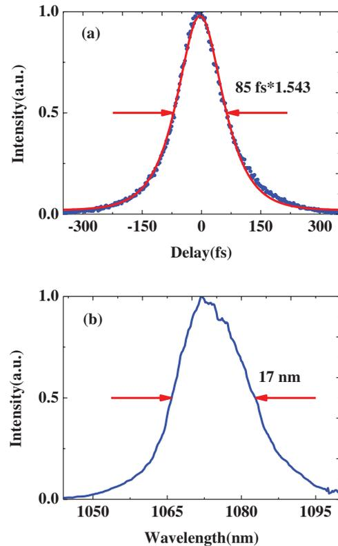
**Figure 2.** (a) Autocorrelation trace of the femtosecond pulses (blue dotted curve) with a  $\text{sech}^2$  fitting (red solid curve). (b) The corresponding spectrum of the mode-locked pulses.
