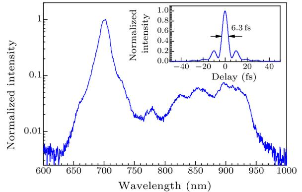
**Fig. 2.** Typical output spectrum of the frequency comb based on the monolithic  $0-f$  scheme. The inset is the Fourier transformation limited pulse duration.
