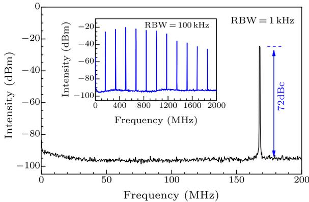
Fig. 4. The RF power spectrum of pulse train detected with a 1 GHz photodetector: with a resolution bandwidth of 1 kHz at the fundamental repetition of 170 MHz and full spectrum up to 1 GHz with 100 kHz resolution.
