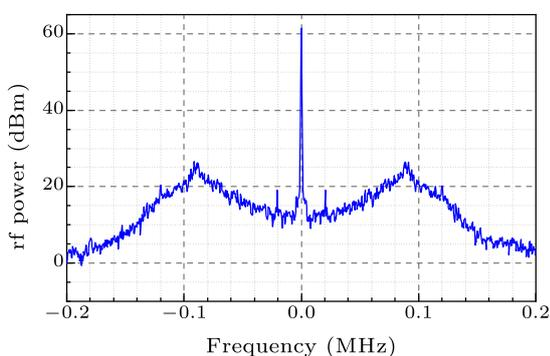
Fig. 6. Noise property of the locked  $f_{\text{ceo}}$  frequency signal directly measured by APD.
