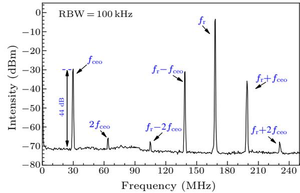
Fig. 5. Free running RF spectrum of  $f_{ceo}$  signal directly measured by APD.
