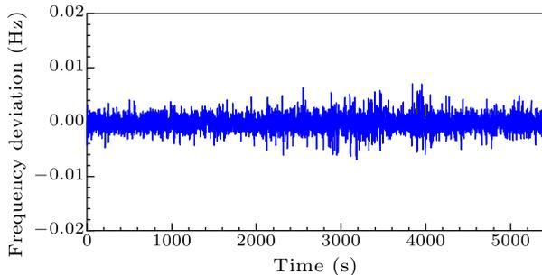
Fig. 8. The locked deviation of the  $f_{\text{ceo}}$  frequency related to the reference frequency (20 MHz). Gate time: 1 s.
