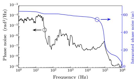
Fig. 7. The phase noise and integral phase of the locked  $f_{\text{ceo}}$  signal. Black curve: the phase noise. Blue curve: the integrated phase noise.
