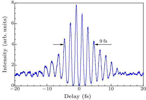
Fig. 3. Interferometric autocorrelation trace of the Ti:sapphire laser oscillator for 9 fs.
