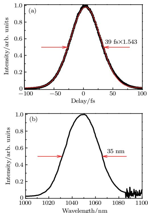
**Fig. 3.** (color online) (a) Autocorrelation trace of the KLM pulses (black dotted curve) with a  $\text{sech}^2$  fitting (red solid curve). (b) The corresponding spectrum.
