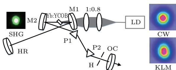
**Fig. 2.** (color online) The experimental setup of the diode-pumped Kerr-lens mode-locked Yb:YCOB femtosecond laser. LD: fiber-coupled diode laser; M1 and M2: plane-concave dichroic mirrors with ROC of 50 mm; HR: high reflection mirror; P1 and P2: SF6 prisms; OC: output coupler; H: pinhole. Right pictures are the beam profiles of the laser at CW and KLM operations and the green beam after M2.
