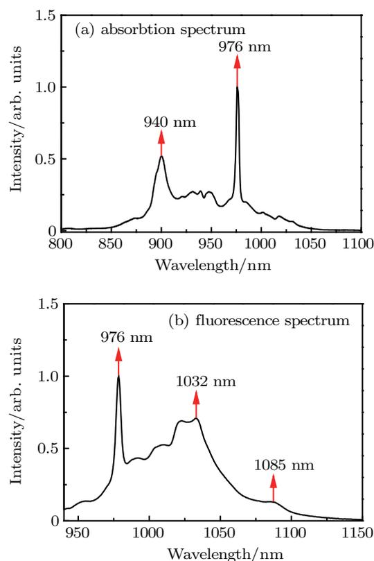
**Fig. 1.** (color online) The absorption spectrum (a) and fluorescence spectrum (b) of the *x*-cut 30 at.%-doped Yb:YCOB crystal at room temperature.
