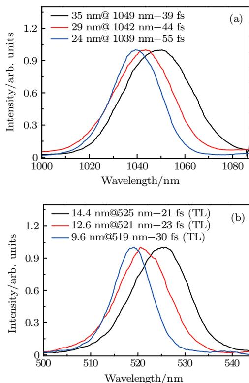
**Fig. 4.** (color online) The wavelength tuning curves of both the near infrared laser (a) and the green laser (b) by means of SHG of the KLM Yb:YCOB laser.
