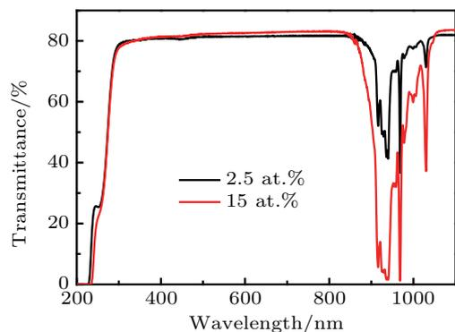
**Fig. 1.** (color online) In-line transmittance curves of 2.5 at.% and 15 at.% Yb:LuAG transparent ceramics (2.7 mm thickness).
