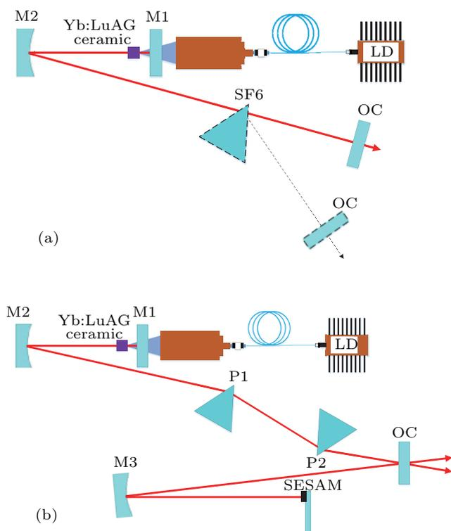
Fig. 4. (color online) Schematic of (a) the continuous wave and (b) the passively mode-locked laser experiment.
