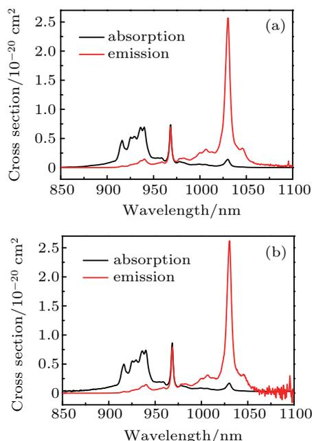
**Fig. 2.** (color online) Absorption and emission cross sections of (a) 2.5 at.% Yb:LuAG and (b) 15 at.% Yb:LuAG transparent ceramics.
