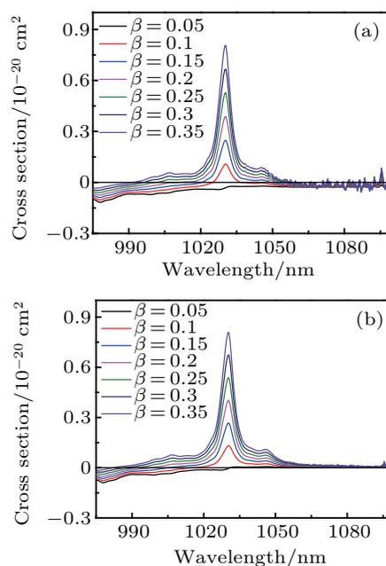
**Fig. 3.** (color online) Gain cross sections of (a) 2.5 at.% Yb:LuAG and (b) 15 at.% Yb:LuAG transparent ceramics.
