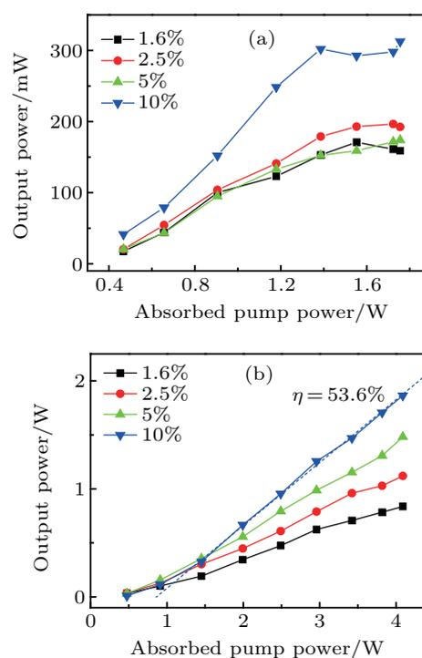
Fig. 5. (color online) Output power of the 2.5 at.% Yb:LuAG ceramic laser (a) and the 15 at.% one (b) as a function of the absorbed pump power with different output couplers.
