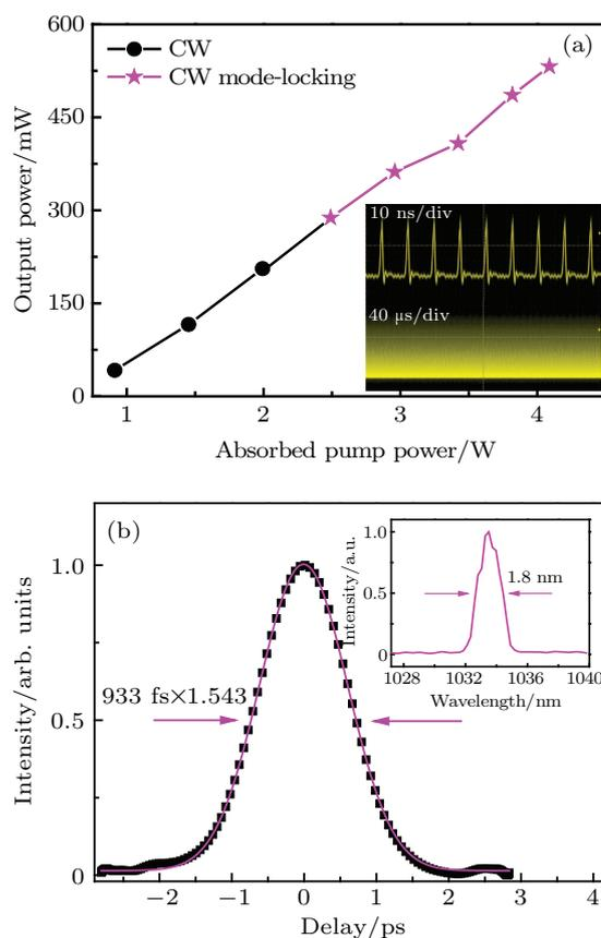
**Fig. 7.** (color online) (a) Output power as a function of the absorbed pump power. Inset shows the pulse trains in 10 ns/div and 40  $\mu$ s/div, respectively. (b) Intensity autocorrelation trace of the mode-locked pulses. The solid square represents the measurement data and the solid curve represents  $\text{sech}^2$ -fitting curve. Inset is the corresponding spectrum.
