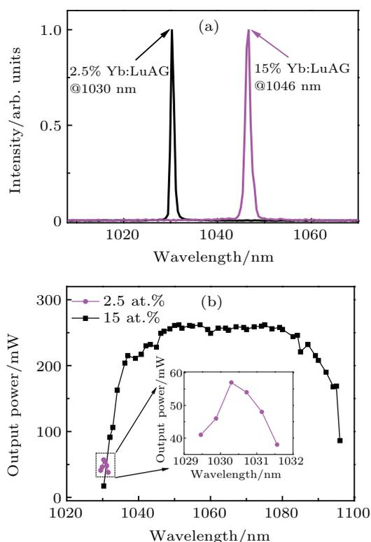
**Fig. 6.** (color online) (a) Continuous wave laser wavelengths for the 2.5 at.% and 15 at.% Yb:LuAG ceramics, and (b) the corresponding wavelength tunability.
