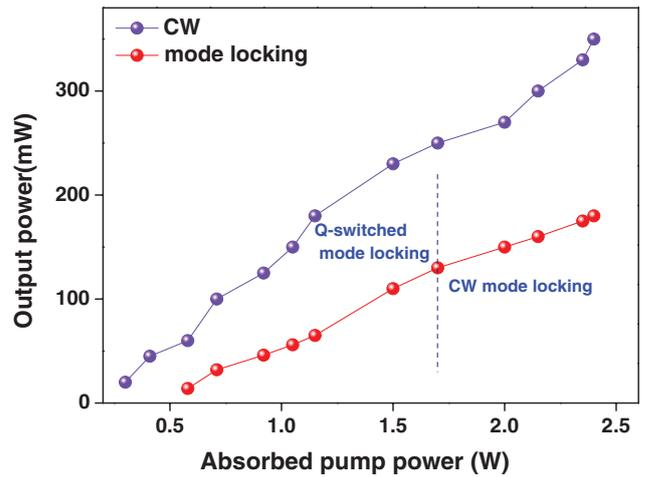
**Figure 3.** CW and passive mode-locked output power versus the absorbed pump power with a 0.8% OC.
