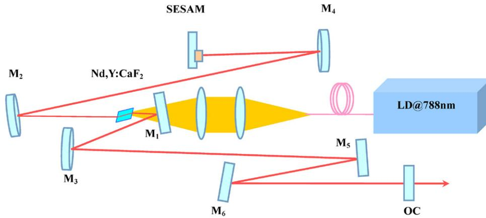
**Figure 1.** Schematic of the experimental setup. LD: laser diode;  $M_1$ : plane dichroic mirror;  $M_2$  and  $M_3$ : concave mirrors with ROC of 200 mm;  $M_4$ : concave mirror with ROC of 300 mm; HR: high reflective mirror;  $M_5$  and  $M_6$ : GTI mirrors; SESAM: semiconductor saturable absorber mirror; OC: output coupler.
