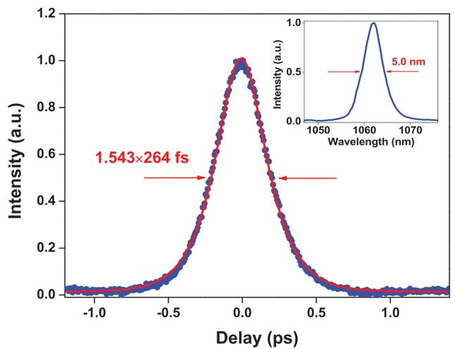
**Figure 4.** Measured intensity autocorrelation trace of the mode-locked pulses (blue dotted) with a sech<sup>2</sup> fitting (red solid). Inset shows the corresponding spectrum.
