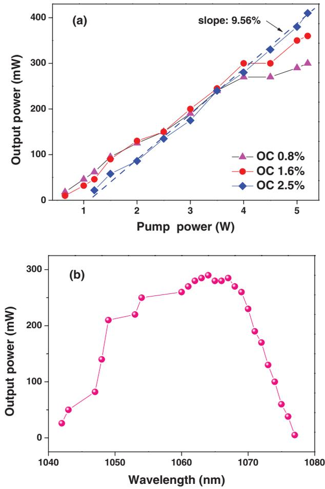
**Figure 2.** (a) CW output power versus the pump power for three OCs of 0.8, 1.6 and 2.5% transmission, respectively. (b) Wavelength tuning curve with an SF6 prism and a 2.5% OC.
