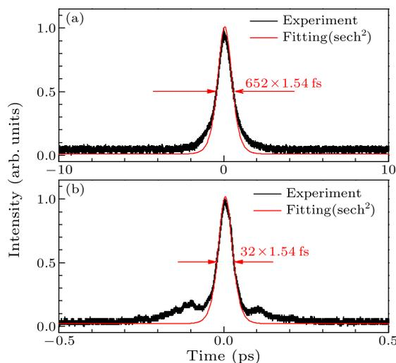
**Fig. 4.** (a) The intensity autocorrelation trace of the pulse train directly from the oscillator (black curve) and  $\text{sech}^2$ -fitting result (red curve). (b) The intensity autocorrelation trace of de-chirped pulse (black curve) and  $\text{sech}^2$ -fitting result (red curve).
