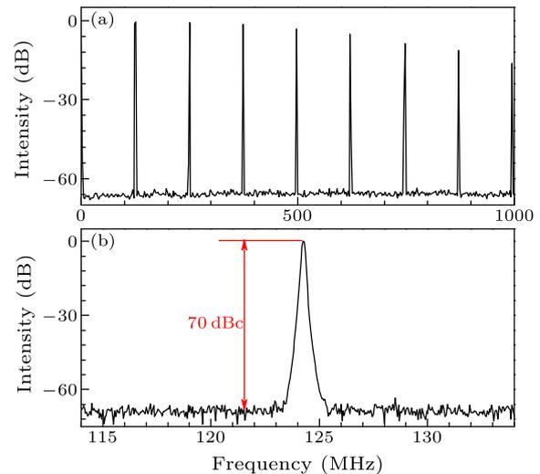
**Fig. 3.** (a) Radio frequency spectrum of 1 GHz wide-span range with a bandwidth resolution of 100 kHz. (b) The rf spectrum of the fundamental frequency, and the signal-to-noise ratio is 70 dBc with a bandwidth resolution of 100 kHz.
