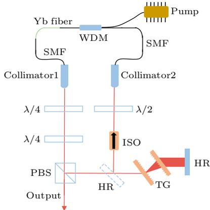
**Fig. 1.** The schematic diagram of the experimental setup: WDM, wavelength division multiplexer; SMF, single mode fiber; PBS, polarization beam splitter; ISO, polarization dependent isolator; TG, transmission grating;  $\lambda/2$ , half-wave plate;  $\lambda/4$ , quarter-wave plate; and HR, high reflection mirror.
