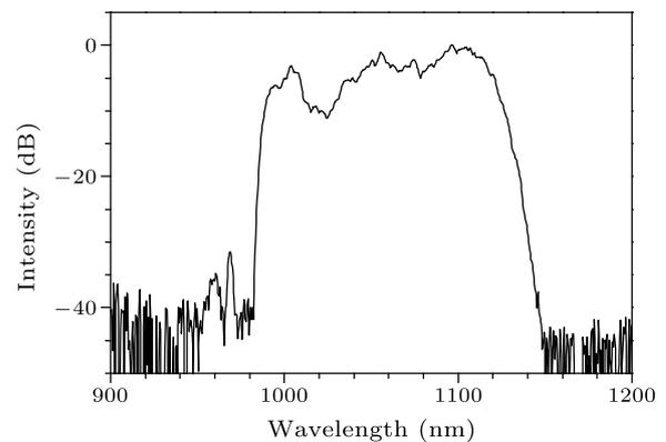
**Fig. 2.** The direct output spectrum from the oscillator with a bandwidth resolution of 1 nm.
